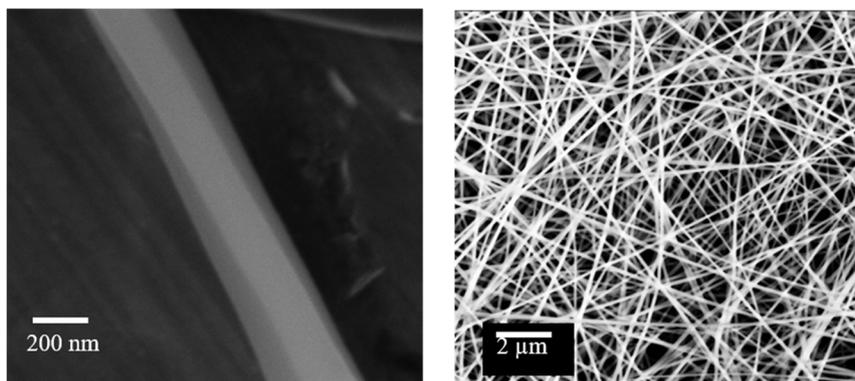
Fig. 1 FESEM images of the synthesized coaxial nanofibers.
