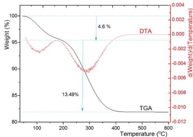
Fig. 9 TGA and DTA curves of CuI@HWSS@CF.
