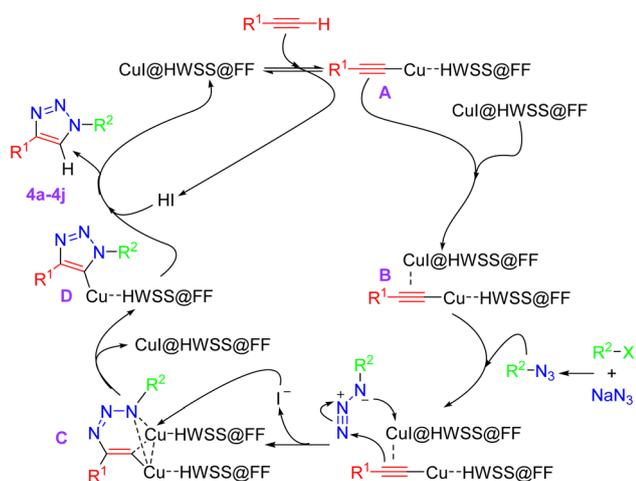
Scheme 2 A plausible mechanism for formation of 1,4-disubstituted-1,2,3-triazoles under catalysis of CuI@HWSS@FF.
