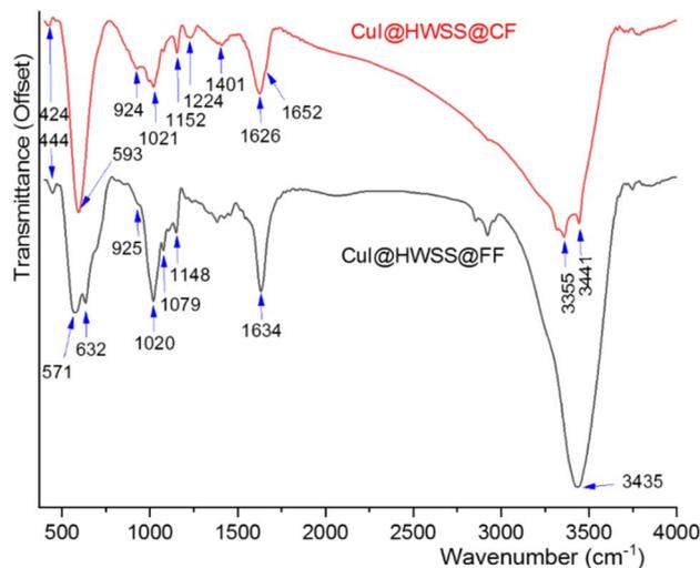
Fig. 12 FT-IR spectra of CuI@HWSS@CF and CuI@HWSS@FF.
