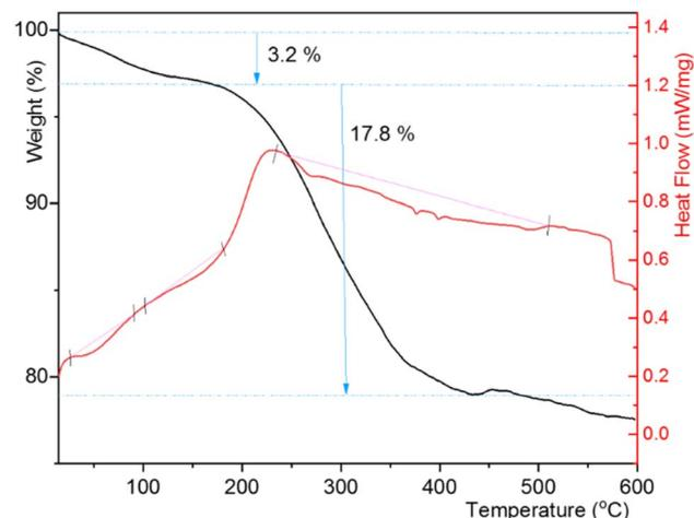
Fig. 10 TGA and DSC curves of CuI@HWSS@FF.
