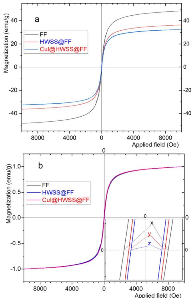
Fig. 8 (a) VSM curves and (b) the normalized VSM curves of CuI@HWSS@FF, HWSS@FF, and FF. The inset displays the coercivities  $y = 56$  Oe,  $z = 50$  Oe and  $x = 72$  Oe for the samples, respectively.
