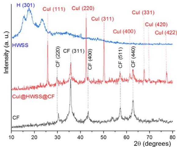
Fig. 1 The XRD-patterns of CF, CuI@HWSS@CF and HWSS.
