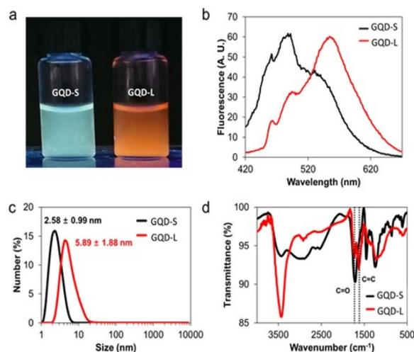
**Fig. 4** GQD-S and GQD-L characterization. (a) Fluorescence images of GQD-S and GQD-L under 365 nm UV light. (b) Emission spectra of GQD-S and GQD-L at 365 nm excitation. (c) Hydrodynamic size distribution. (d) FT-IR spectra.
