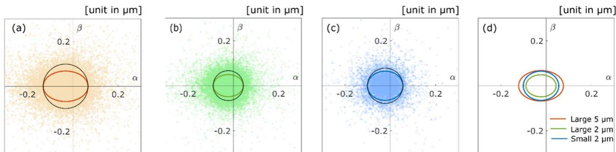
Fig. 6 Scatter diagrams for the diffusion anisotropy of the aggregates with diameter  $d$  for the columns with pore size  $126d$  (orange) (a) and  $8d$  (green) (b), and the aggregates with diameter  $0.2d$  for the column with pore size  $8d$  (blue) (c). The coloured lines of ellipses are the radii of gyrations, and the black solid lines are the circles for which radii are equal to the radius of gyrations of the  $\alpha$  axis. (d) Coloured lines of ellipses in (a)–(c) are overlaid.
