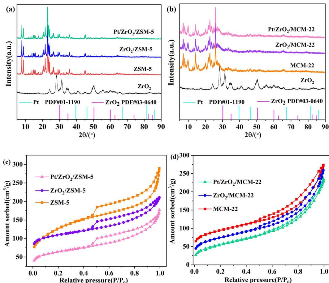
Fig. 1 XRD patterns (a and b) and N<sub>2</sub> adsorption-desorption isotherms (c and d) of Pt catalysts.
