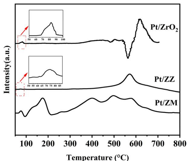
Fig. 4 H<sub>2</sub>-TPR profiles of Pt catalysts.
