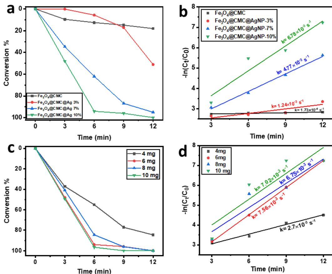
Fig. 4 (a) Plots of conversion vs. reaction time and (b) plots of  $-\ln(C_t/C_0)$  vs. reaction time of 4-NP with  $Fe_3O_4/CMC$ ,  $Fe_3O_4/CMC-Ag-3\%$ ,  $Fe_3O_4/CMC-Ag-7\%$  and  $Fe_3O_4/CMC-Ag-10\%$ . (c) Plots of conversion vs. reaction time and (d) plots of  $-\ln(C_t/C_0)$  vs. reaction time of 4-NP with  $Fe_3O_4/CMC$ ,  $Fe_3O_4/CMC-Ag-3\%$ ,  $Fe_3O_4/CMC-Ag-7\%$  and  $Fe_3O_4/CMC-Ag-10\%$  with different dosages.
