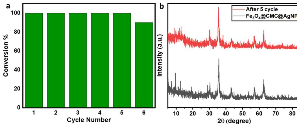
Fig. 6 (a) The reusability cycles of Fe<sub>3</sub>O<sub>4</sub>/CMC-Ag-10%. (b) XRD patterns of Fe<sub>3</sub>O<sub>4</sub>/CMC-Ag-10% before and after 5 cycles.
