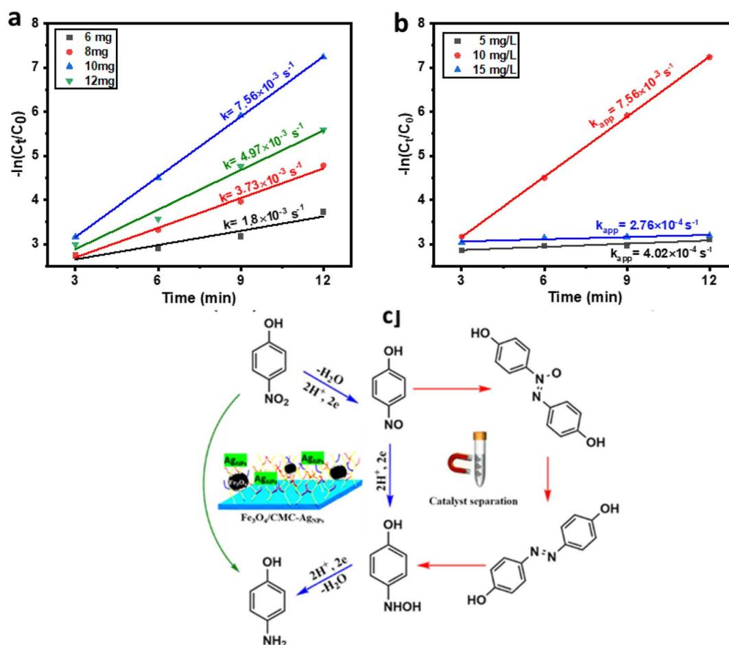
Fig. 5 (a) Plots of  $-\ln(C_t/C_0)$  vs. reaction time of  $NaBH_4$  optimization. (b) plots of  $-\ln(C_t/C_0)$  vs. reaction time of concentration optimization of 4-NP. (c) Plausible mechanism for 4-NP reduction to 4-AP.
