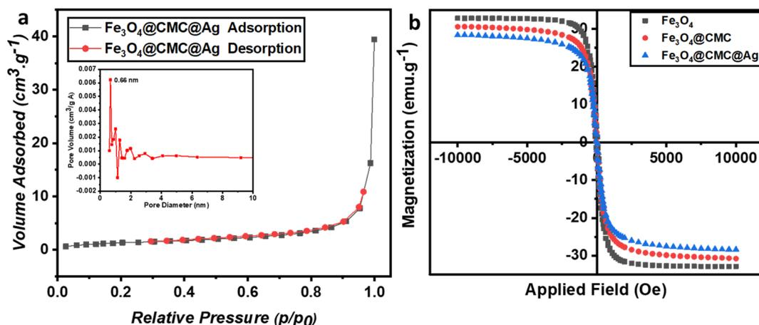
Fig. 3 (a) N<sub>2</sub> adsorption–desorption isotherms and pore diameter of Fe<sub>3</sub>O<sub>4</sub>/CMC-Ag-7%. (b) Magnetic hysteresis loops for pristine Fe<sub>3</sub>O<sub>4</sub>, Fe<sub>3</sub>O<sub>4</sub>/CMC, and Fe<sub>3</sub>O<sub>4</sub>/CMC-Ag-7%.
