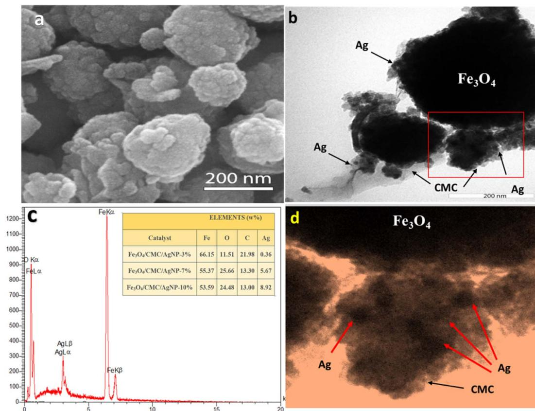
Fig. 2 (a) SEM image of Fe<sub>3</sub>O<sub>4</sub>/CMC-Ag-7%. (b and d) TEM image of Fe<sub>3</sub>O<sub>4</sub>/CMC-Ag-7%. (c) EDX spectrum of Fe<sub>3</sub>O<sub>4</sub>/CMC-Ag-7%.
