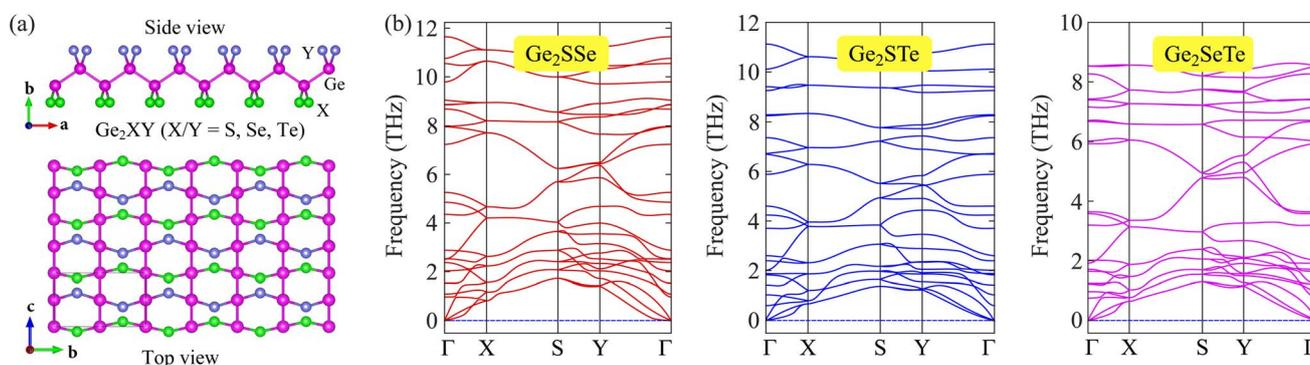
Fig. 1 Crystal structures (a) and phonon dispersions (b) of Janus Ge<sub>2</sub>XY (X/Y = S, Se, and Te; X ≠ Y) monolayers.
