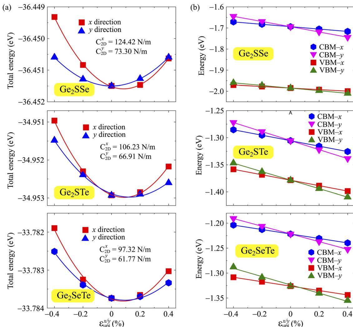
Fig. 6 The uniaxial strain dependence of (a) the total energy shifts and (b) band-edge positions of  $\text{Ge}_2\text{XY}$  structures.
