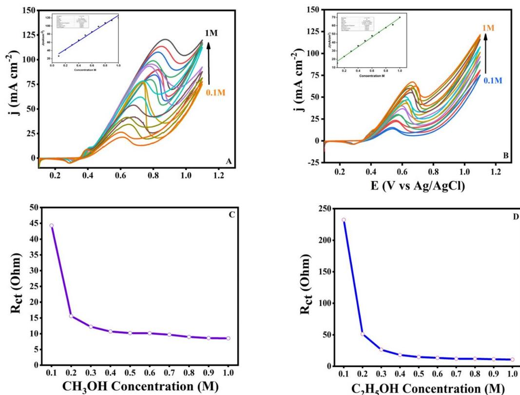
Fig. 10 Curves of cyclic voltammograms of CP@Ni@NATPhos/Ni at a rate of 50 mV s<sup>-1</sup> in a 1 M NaOH solution containing concentrations of methanol (A) and ethanol (B). Charge resistance transfer dependency determined from impedance spectroscopy results at different methanol (C) and ethanol (D) concentrations.
