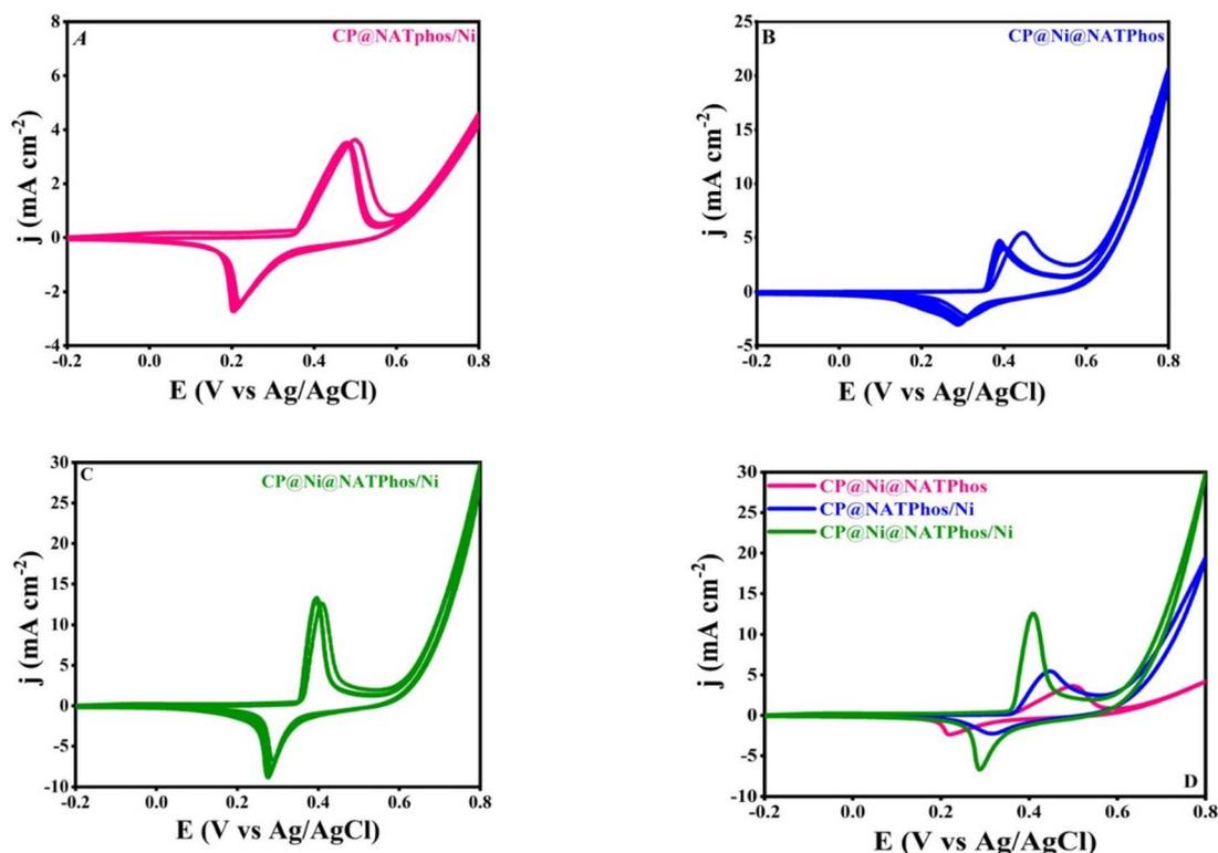
Fig. 6 Successive CVs for CP@NATPhos/Ni (A), CP@Ni@NATPhos (B), and CP@Ni@NATPhos/Ni (C) in solution containing 1 M of NaOH at a scan rate of  $50 \text{ mV s}^{-1}$ . Only representative cycles are shown of total of 10 cycles. (D) Comparison of the 10th cycle of all electrodes.
