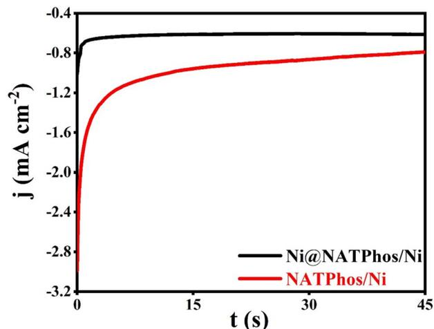
Fig. 5 Electrodeposition of the nickel nanoparticles at  $E = -0.5$  V for 45 s: (a) Ni@NATPhos/Ni and (b) NATPhos/Ni.
