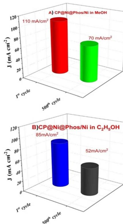
Fig. 12 The first and 500th scans for CP@Ni@Phos/Ni in (A) 1 M NaOH + 1 M CH<sub>3</sub>OH solution, (B) CP@Ni@Phos/Ni after 500 cycles in 1 M NaOH + 1 M C<sub>2</sub>H<sub>5</sub>OH solutions.
