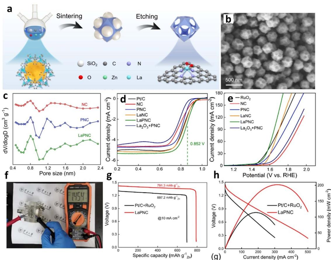
**Fig. 6** (a) Formation process of LaPNC. (b) SEM image of LaPNC. (c) Micropore size analysis of LaPNC and its comparison samples. (d) LSV curves for various materials as ORR catalysts at 1600 rpm and (e) as OER catalysts. (f) Open-circuit voltage of LaPNC. (g) Discharge polarization and power density curves, and (h) specific capacities at 10 mA cm<sup>-2</sup> for ZABs with LaPNC and Pt/C + RuO<sub>2</sub> air cathodes. Reproduced with permission from ref. 90 Copyright 2022, Elsevier.
