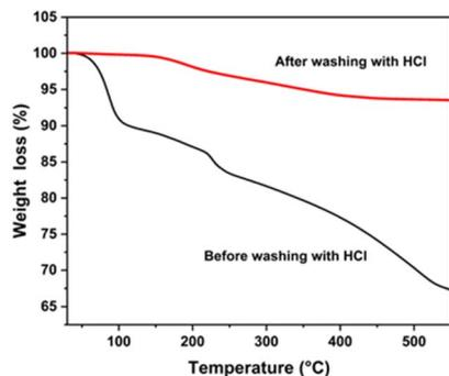
Fig. 9 TGA spectrum of CZTS NPs synthesized at 240 °C for 30 minutes: before washing with HCl (black spectrum) and after washing with HCl (red).
