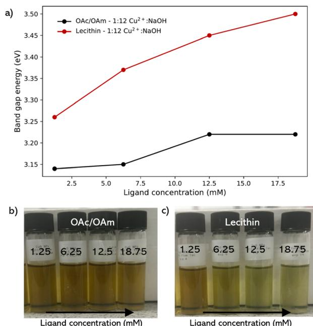
Fig. 4 (a) corresponding band gap energies of the CuO NP colloidal solutions synthesized using OAc/OAm binary and soy-lecithin flow conditions. Photographs of CuO NPs synthesized in flow at 1 : 12  $\text{Cu}^{2+}$  : NaOH ratio using (b) oleic acid (OAc) and oleylamine (OAm) binary mixture, and (c) soy-lecithin zwitterion at various molar concentrations.
