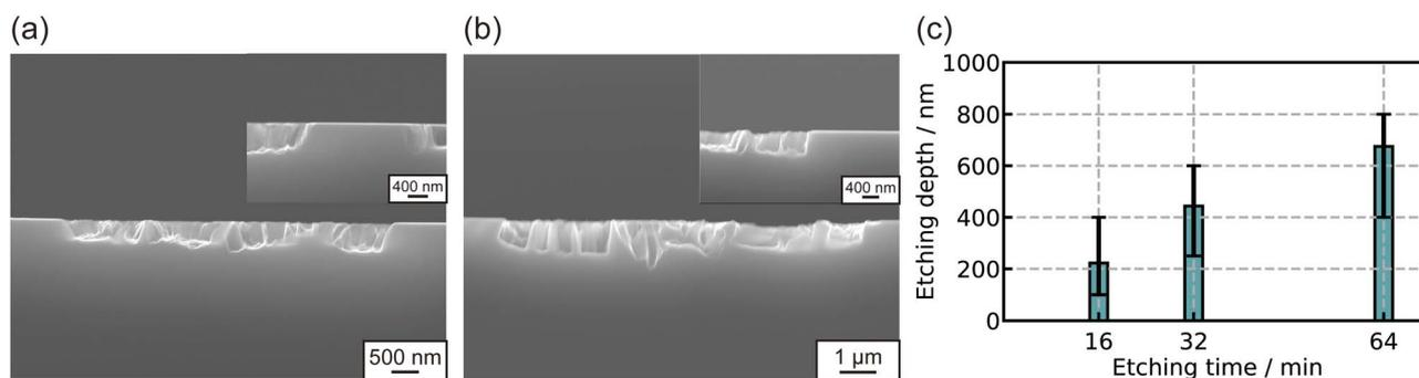
Fig. 7 Cross-sectional SEM images of the etched silicon loaded with GO sheets under  $-3.0$  V for (a) 32 min, and (b) 64 min, respectively. Insets show higher magnification. (c) The relationship between the etching time and the etching depth under  $-3.0$  V.
