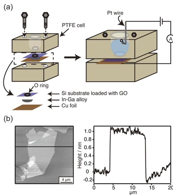
Fig. 1 (a) Schematic illustration of the experimental setup of electrochemically GO-assisted silicon etching. (b) An AFM topographic image and cross-sectional profile along the line after spin-coating the GO dispersion on a silicon substrate.
