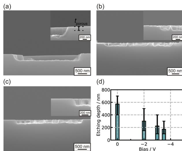
Fig. 3 Cross-sectional SEM images of the silicon loaded with GO sheets after 16 min etching under (a)  $-2.0$  V, (b)  $-3.0$  V, (c)  $-3.5$  V at room temperature. Insets show higher magnification. (d) The relationship between the applied bias and the etching depth after etching for 16 min.
