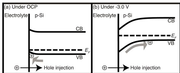
Fig. 6 Schematic band diagrams showing the mechanism of etching. (a) shows the interface between the electrolyte and the bare silicon under OCP, whereas (b) shows under the  $-3.0$  V. CB, VB, and  $E_F$  are the conduction band edge, the valence band edge, and the Fermi level of the p-type silicon, respectively.
