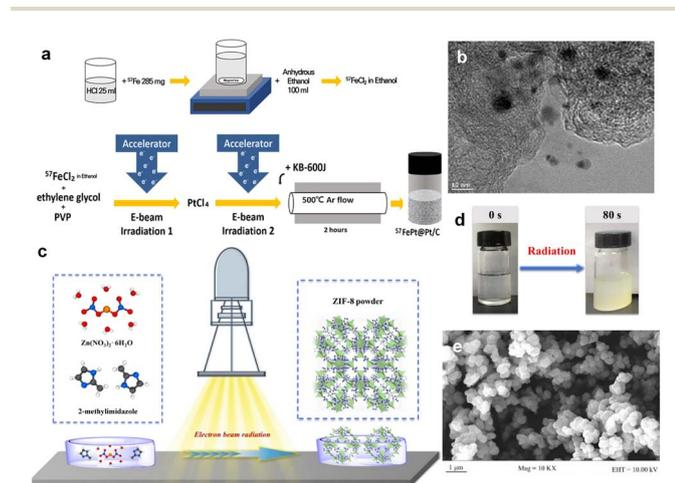
Fig. 4 (a) Schematic illustration of the synthesis of  $^{57}\text{FePt}@Pt/C$  via electron-beam irradiation. (b) TEM image of  $^{57}\text{FePt}@Pt/C$ . Copyright 2023 Wiley-VCH. (c) The synthesis setup of ZIF-8 via electron beam radiation. (d) The photo of ZIF-8 synthesized at an absorbed dose of 50 kGy. (e) SEM image of ZIF-8 at an absorbed dose of 50 kGy.<sup>54,55</sup> Copyright 2022, Wiley-VCH.
