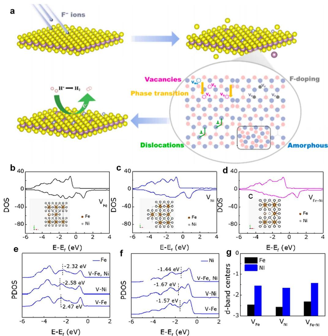
Fig. 6 (a) Schematic illustration of the irradiation process of MoS<sub>2</sub> structure evolution. Copyright 2023 American Chemical Society. DOS of (b) FeNi<sub>3</sub>-V<sub>Fe</sub>, (c) FeNi<sub>3</sub>-V<sub>Ni</sub>, and (d) FeNi<sub>3</sub>-V<sub>Fe-Ni</sub>. PDOS of (e) Fe and (f) Ni atoms under three different structures. (g) Changes in the d-band center. Copyright 2024 Elsevier Ltd.
