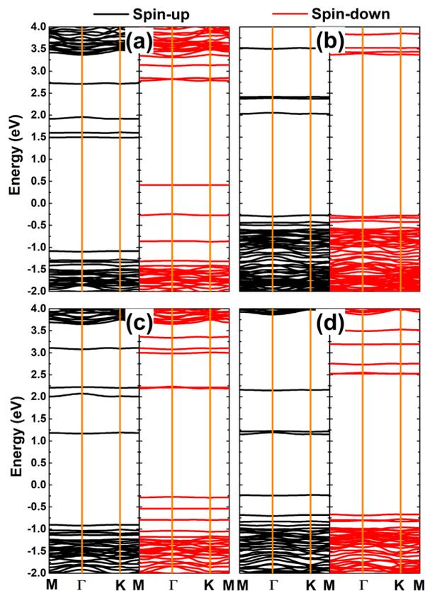
Fig. 8 Spin-polarized band structure (the Fermi level is set to 0 eV) of the HfO<sub>2</sub> monolayer doped with (a) MnB, (b) MnC, (c) FeB, and (d) FeC pair atoms.
