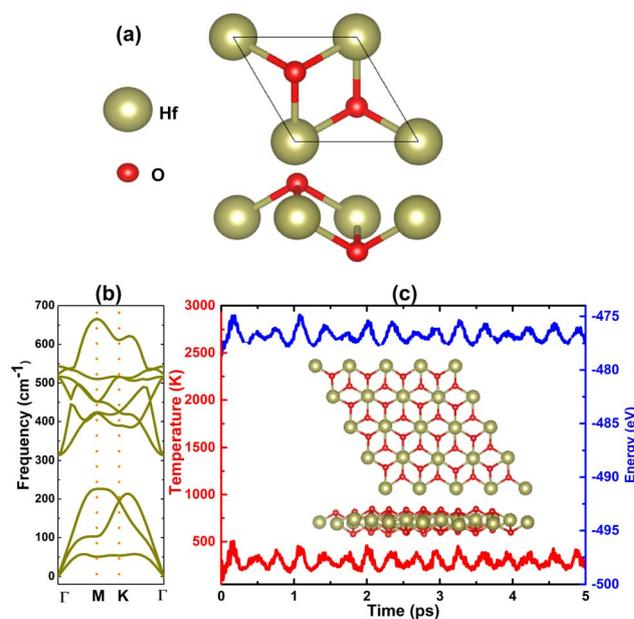
Fig. 1 (a) Atomic structure in a unit cell, (b) phonon dispersion curves, and (c) AIMD simulations at 300 K (inset final atomic structure in the 4 × 4 × 1 supercell of the HfO<sub>2</sub> monolayer).
