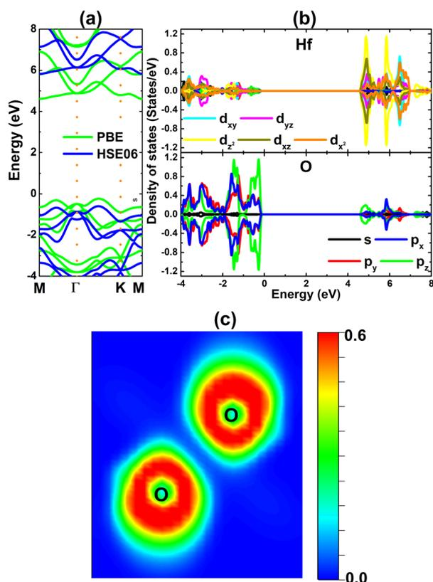
Fig. 2 (a) Electronic band structure (the Fermi level is set to 0 eV), (b) projected density of states, and (c) electron localization function of the HfO<sub>2</sub> monolayer.
