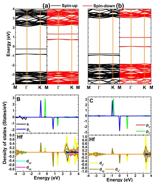
Fig. 6 Spin-polarized band structure (the Fermi level is set to 0 eV) and projected density of states of B/C impurities and their neighboring Hf atoms in (a) B- and (b) C-doped HfO<sub>2</sub> monolayers.
