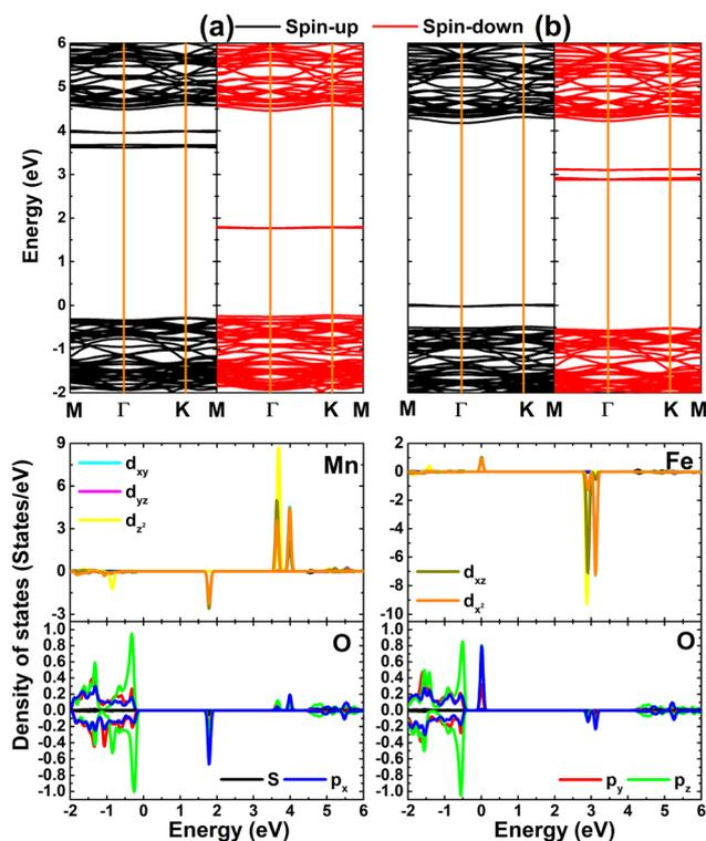
Fig. 4 Spin-polarized band structure (the Fermi level is set to 0 eV) and projected density of states of Mn/Fe impurities and their neighboring O atoms in (a) Mn- and (b) Fe-doped HfO<sub>2</sub> monolayers.
