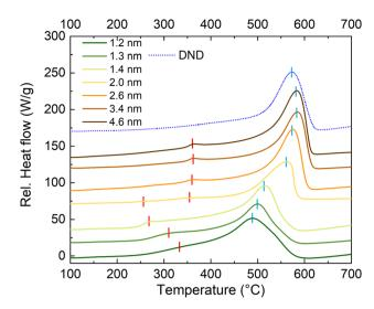
Fig. 1 DSC data of the ND samples as a function of ND size. DSC trace of DND sample (dotted blue line) is shown for comparison. The peaks related to the oxidation of  $C-H_x$  bonds and of the combustion are highlighted by short red and pale blue lines, respectively.
