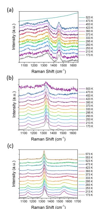
Fig. 7 Temperature-dependent Raman spectra of 1.2 nm (a), 2.0 nm (b) and 4.6 nm (c) samples.
