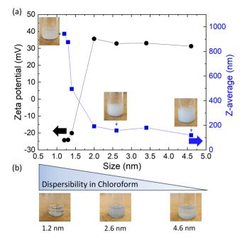
Fig. 5 Z-Average (blue) and zeta potential (black) of the BU\_HPHT NDs as function of size obtained by DLS and zeta potential measurements. Selected samples are accompanied by photographs of their dispersions (a). BU\_HPHT NDs dispersions of selected samples in chloroform with an indicated decrease in dispersibility with increasing
