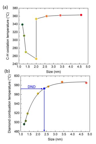
Fig. 2  $C-H_x$  oxidation (a) and ND combustion temperatures (b) as a function of size. The line in (a) is to guide the eye. The data in (b) were fitted by an asymptotic function. The point of DND was placed on the curve taking the DND oxidation temperature to derive a hypothetic ND size that would correspond to "monocrystalline DND".
