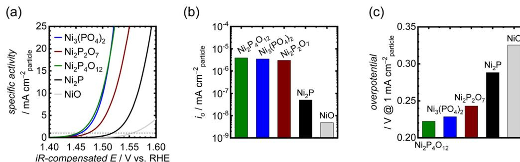
Fig. 3 (a) Polarization curves showing OER-specific activities for the Ni-based phosphates, NiO, and Ni<sub>2</sub>P in 1 M KOH. (b) *i*<sub>0</sub> values for the OER of the Ni-based phosphates, NiO, and Ni<sub>2</sub>P. (c) Comparison of their OER overpotentials at 1 mA cm<sub>particle</sub><sup>-2</sup>.
