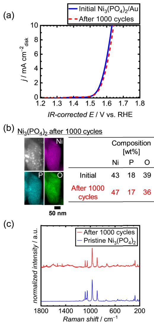
Fig. 5 (a) Polarization curves of  $\text{Ni}_3(\text{PO}_4)_2/\text{Au}$  after 1000 repeated potential cycles between 1.2 and 1.7 V *vs.* RHE in 1 M KOH. (b) STEM-EDX image and (c) Raman spectrum of  $\text{Ni}_3(\text{PO}_4)_2/\text{Au}$  after 1000 potential cycles.
