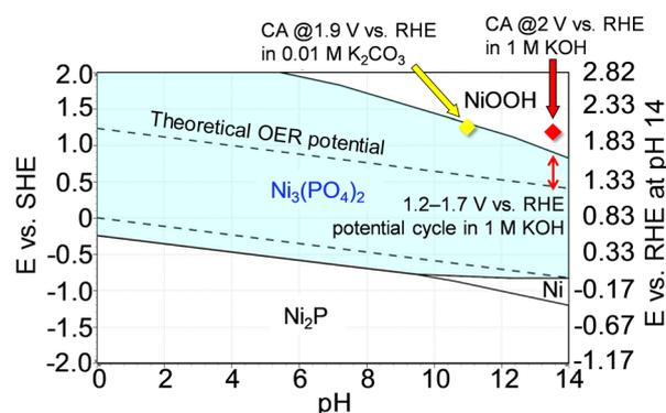
Fig. 6 Pourbaix diagram of the Ni–P–H<sub>2</sub>O system at 298.15 K with the assumed concentration of soluble species and pressure set at 1.0 M and 1.0 bar, respectively. The scale on the right axis represents the RHE potential at pH 14. The converted potentials at pH 13.7 (1 M KOH) and 10.9 (0.01 M K<sub>2</sub>CO<sub>3</sub>) were calculated using the equation  $E_{\text{RHE}} = E_{\text{SHE}} + 0.0592 \times \text{pH}$ .<sup>66</sup>
