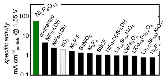
Fig. 4 Comparison of the OER-specific activity of Ni<sub>2</sub>P<sub>4</sub>O<sub>12</sub> in alkaline media with the state-of-the-art crystalline nonprecious metal-based catalysts, BSCF, and IrO<sub>2</sub>. Further details of the cited literature are presented in the ESI.<sup>†</sup>
