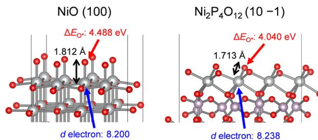
Fig. 9 DFT-optimized surface slab models of NiO (100) and Ni<sub>2</sub>P<sub>4</sub>O<sub>12</sub> (10  $\bar{1}$ ) showing the Ni–O\* bond length, the number of d electrons in the Ni atoms, and  $\Delta E_{O^*}$ . The gray, purple, and red spheres represent Ni, P, and O atoms, respectively.
