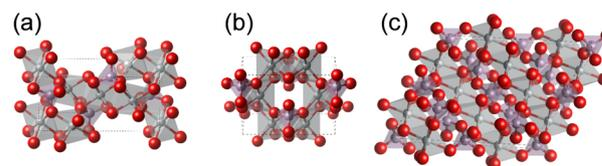
Fig. 1 Crystal structures of Ni-based phosphates. (a) Ni<sub>3</sub>(PO<sub>4</sub>)<sub>2</sub>, (b) Ni<sub>2</sub>P<sub>2</sub>O<sub>7</sub>, and (c) Ni<sub>2</sub>P<sub>4</sub>O<sub>12</sub>. The gray, purple, and red spheres represent Ni, P, and O atoms, respectively.
