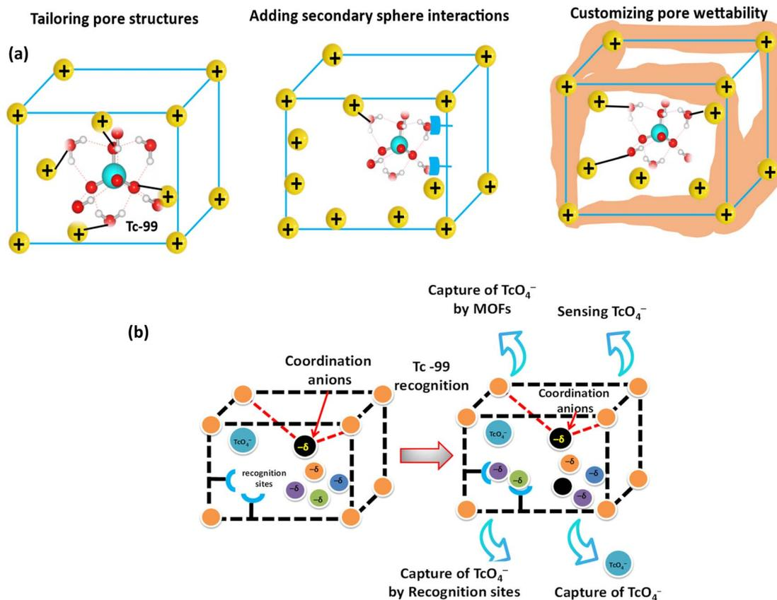
Fig. 1 (a)  $^{99}\text{TcO}_4^-$  adsorption efficiency can be increased by the following methods: designing pore architectures to boost charge density; adding secondary sphere interactions to fortify binding; and regulating pore wettability to enhance binding affinity. (b) Recognition and capture of  $^{99}\text{TcO}_4^-$  using MOFs.
