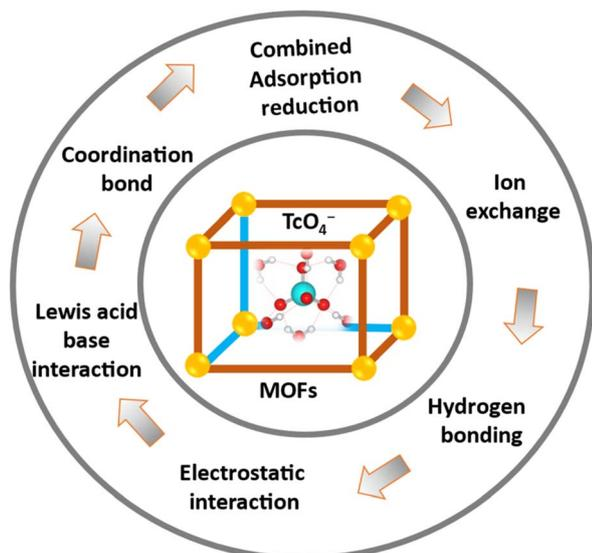
Fig. 14 Mechanisms of  $\text{TcO}_4^-/\text{ReO}_4^-$  ion extraction with MOFs.
