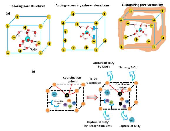
Fig. 1 (a) 99TcO<sub>4</sub> adsorption efficiency can be increased by the following methods: designing pore architectures to boost charge density; adding secondary sphere interactions to fortify binding, and regulating pore wettability to enhance binding affinity. (b) Recognition and capture of  $^{99}\text{TcO}_4^-$  using MOFs.
