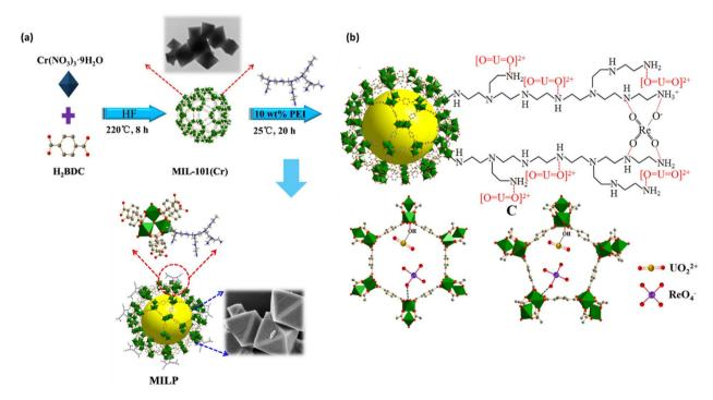
Fig. 7 (a) The synthesis approach flowchart for MILP MOF composites. The figure is reproduced from ref. 65 with permission from Elsevier. (b) Possible host–guest interactions between  $UO_2^{2+}$  and  $ReO_4^{-}$  with the MIL-101(Cr) cavities and schematic depiction of the interaction between  $UO_2^{2+}$  and  $ReO_4^-$  with PEI. The figure is reproduced from ref. 65 with permission from Elsevier.
