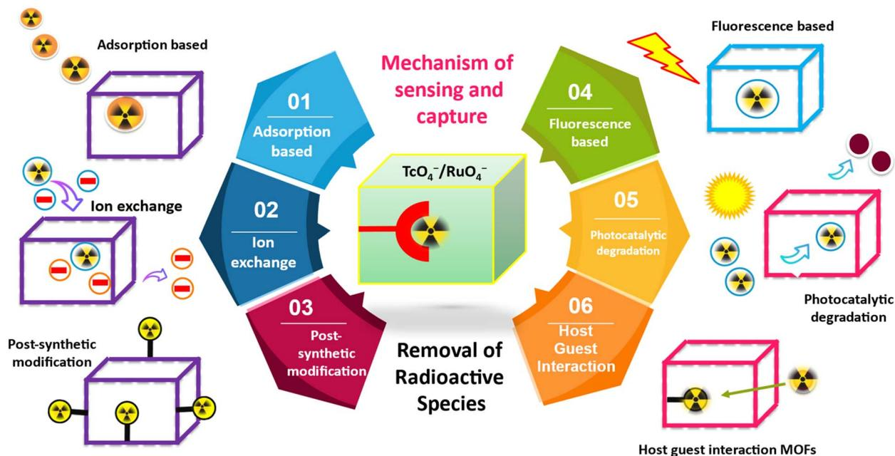
Fig. 3 MOF-based material for removal of  $\text{TcO}_4^-/\text{RuO}_4^-$ .
