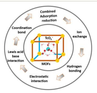
Fig. 14 Mechanisms of  $TcO_4^-/ReO_4^-$  ion extraction with MOFs.
