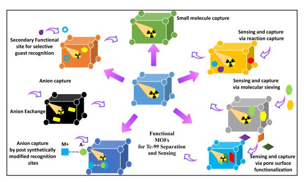
Fig. 2 Different mechanisms of TcO<sub>4</sub><sup>-</sup> adsorption using functionalized MOFs.
