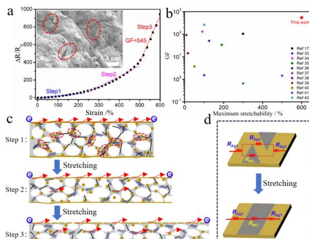
**Fig. 4** (a) The resistance change–strain curve of the strain sensor and SEM image of the AMGT fiber at 550% strain. (b) Comparison of performance with other fiber strain sensors. (c) Schematic of the sensing mechanism of the strain sensor at different stages. (d) Resistance model of the sensor under different strains.
