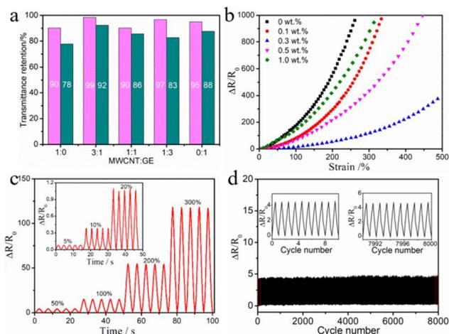
**Fig. 3** (a) Statistics of the retention rate of ultraviolet-visible transmittance of different fillers in DMF. (b) The resistance change–strain curves of AMGT conductive fibers with different filler contents. (c) The resistance change–time curves of the strain sensor under different loading and unloading stretches. (d) Durability test of the sensor under repeated 0–50% strains in 8000 cycles.
