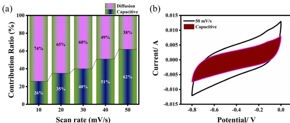
Fig. 5 (a) Contribution ratio of capacitance to total charge for FeS- $W_{18}O_{49}$  from  $10 \text{ mV s}^{-1}$  to  $50 \text{ mV s}^{-1}$ ; (b) contribution of the surface capacitance of FeS- $W_{18}O_{49}$  at  $50 \text{ mV s}^{-1}$ .
