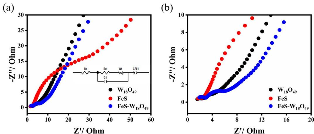
Fig. 6 (a) Nyquist impedance plot comparing the electrochemical impedance of  $W_{18}O_{49}$ , FeS, and the FeS- $W_{18}O_{49}$  composite, accompanied by an inset showing the equivalent circuit model. (b) Enlarged view of the high-frequency region for detailed analysis.
