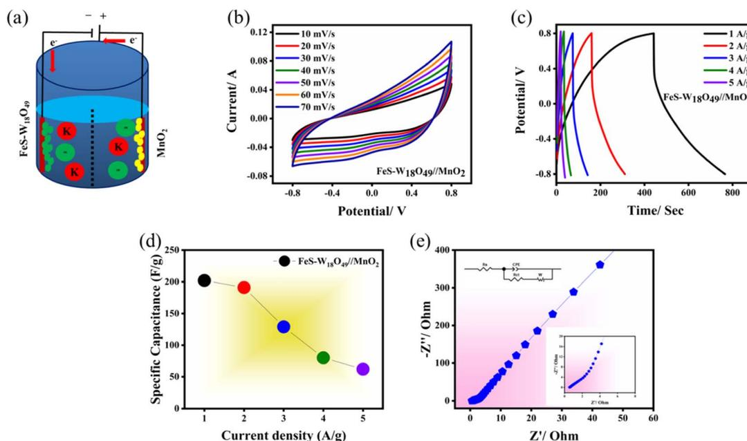
**Fig. 8** Characteristics of the FeS–W<sub>18</sub>O<sub>49</sub>||MnO<sub>2</sub> ASC: (a) schematic illustration of the FeS–W<sub>18</sub>O<sub>49</sub>||MnO<sub>2</sub> device, (b) CV curve at 1.6 V, (c) GCD curves at 1–5 A g<sup>-1</sup>, (d) specific capacitance as a function of current density, and (e) EIS plot.
