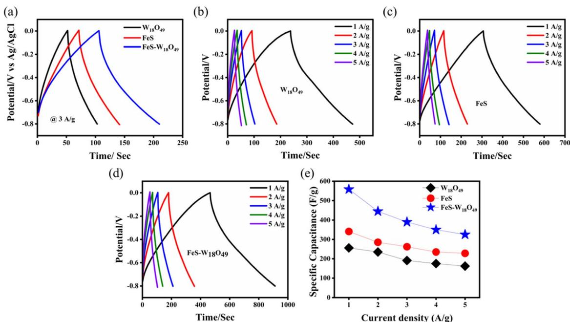
Fig. 7 (a) Comparative galvanostatic charge-discharge (GCD) performance of all electrodes at a current density of  $3 \text{ A g}^{-1}$ , GCD curves of (b)  $W_{18}O_{49}$ , (c) FeS, (d) FeS- $W_{18}O_{49}$  composite electrodes, and (e) specific capacitance values of all the prepared electrodes.
