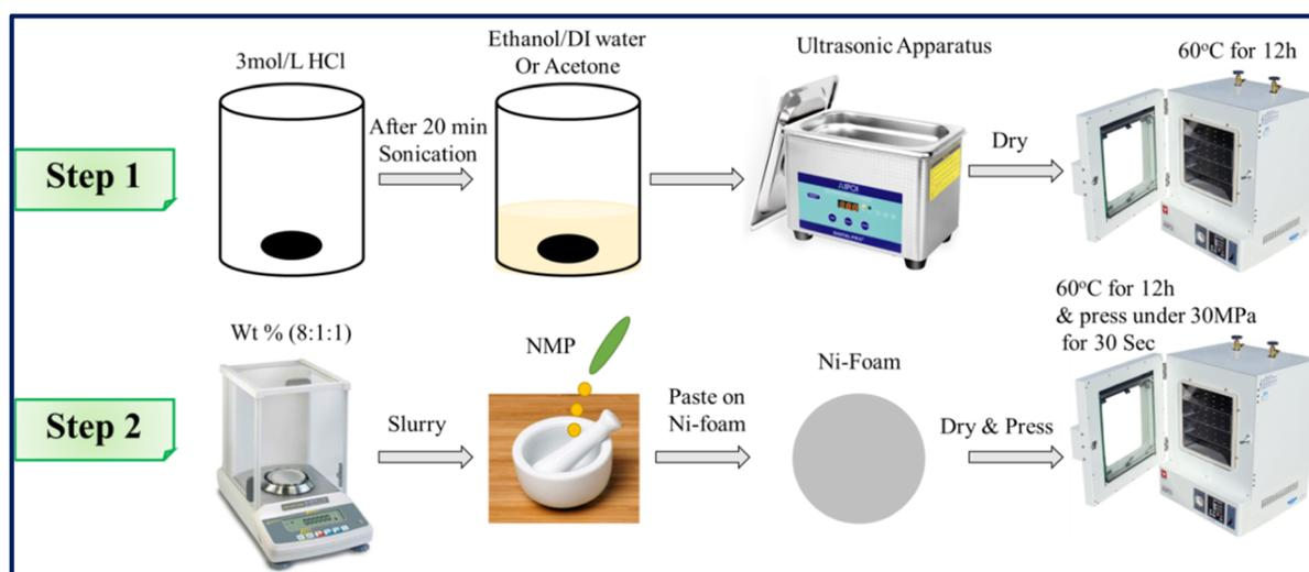
Fig. 1 Schematic diagram of preparation of electrodes.
