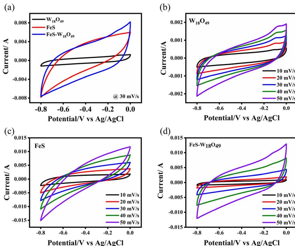
Fig. 4 (a) Cyclic voltammetry (CV) curves of  $W_{18}O_{49}$ , FeS and the FeS- $W_{18}O_{49}$  nanocomposite at a scan rate of  $30 \text{ mV s}^{-1}$ , and (b)  $W_{18}O_{49}$ , (c) FeS, and (d) the FeS- $W_{18}O_{49}$  composite at various scan rates.
