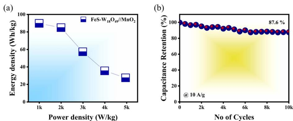
Fig. 9 (a) Ragone plot illustrating the energy and power density relationship of the FeS-W<sub>18</sub>O<sub>49</sub>||MnO<sub>2</sub> ASC. (b) Long-term cycling stability test at a high current density of 10 A g<sup>−1</sup>.
