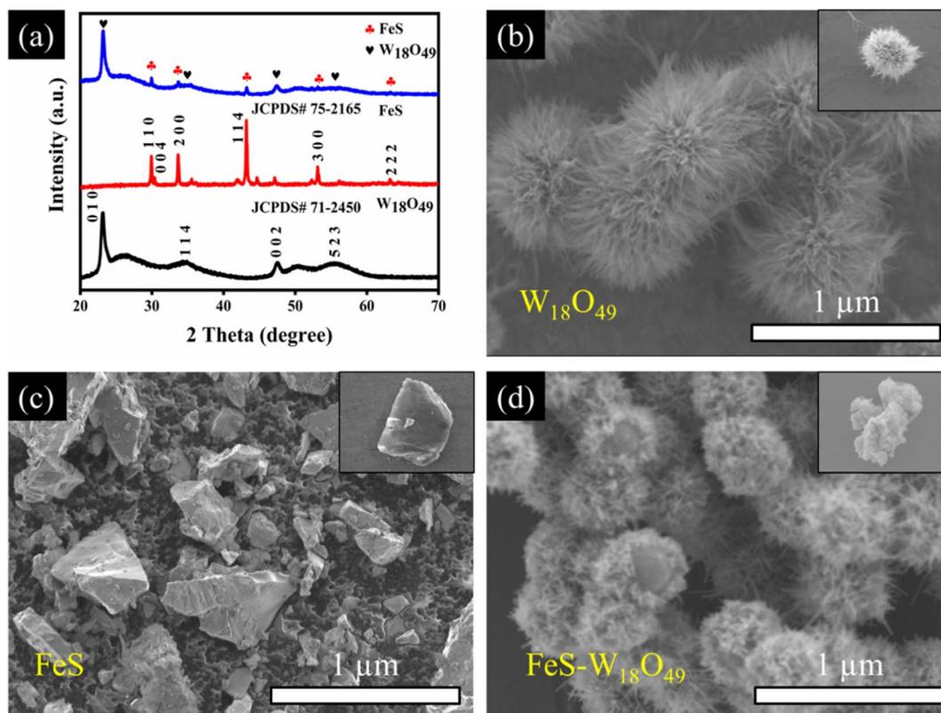
Fig. 2 XRD patterns of  $W_{18}O_{49}$ , FeS, and the FeS- $W_{18}O_{49}$  nanocomposite (a), accompanied by SEM images showcasing the morphology of (b)  $W_{18}O_{49}$ , (c) FeS, and (d) the FeS- $W_{18}O_{49}$  nanocomposite.
