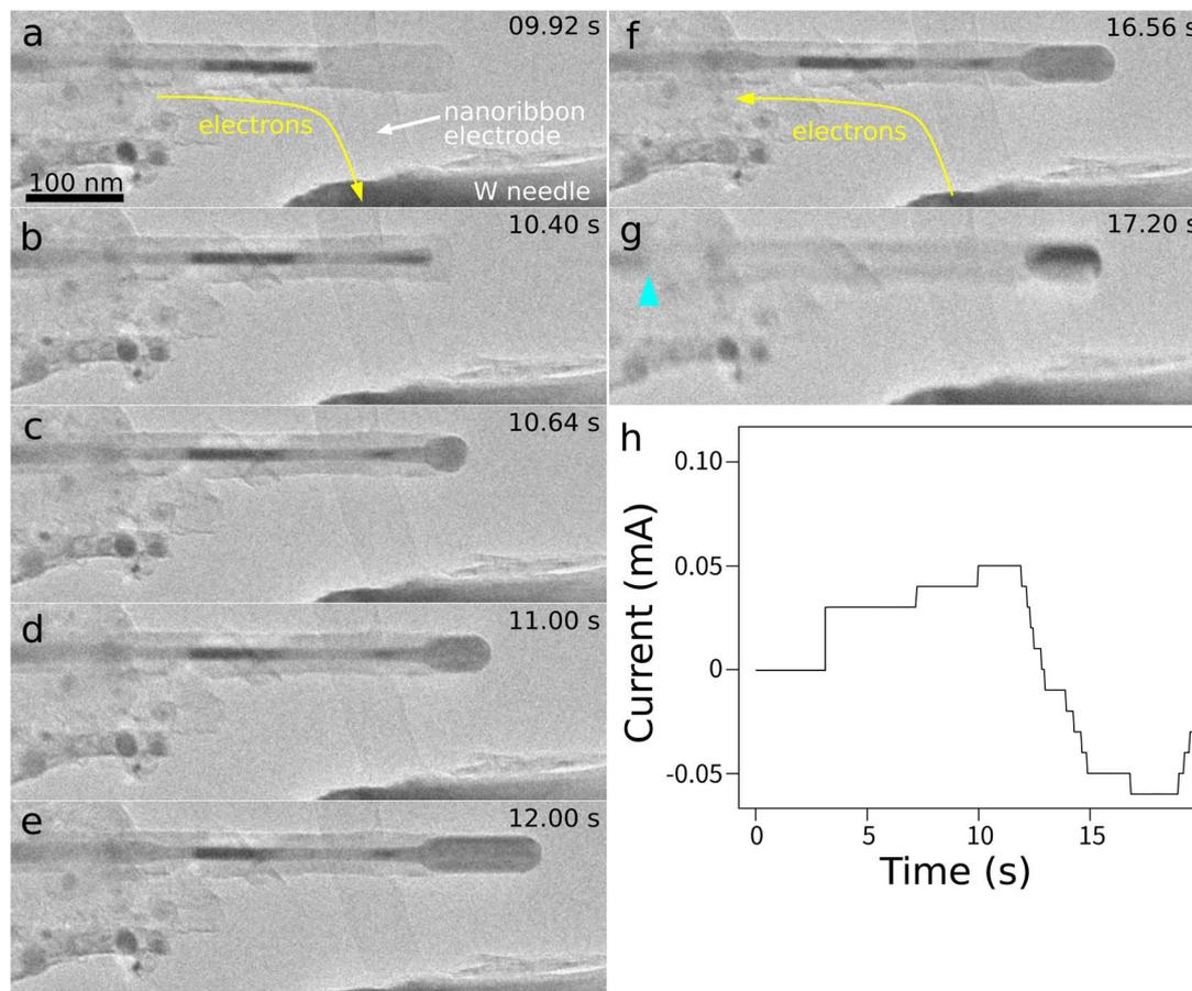
Fig. 3 (a–g) *In situ* TEM images of electromigration manipulation of a Co nanorod filler. The Co filler was first pushed out of the MWCNT and then pulled into the MWCNT when the direction of electron flow was reversed. The filler split into two portions at the shoulder. The blue arrow head in (g) indicates the position of the right end of the left portion. (h) Plot of current as a function of time. The direction of electron flow was reversed at around 13.0 s (ESI movie† SM3 available).
