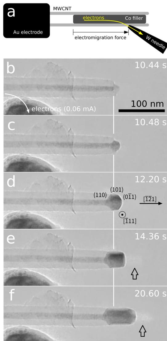
**Fig. 1** (a) Schematic illustration of experimental setup. (b–f) *In situ* TEM images of electromigration manipulation of a Co nanorod filler. The Co filler was pushed out of the MWCNT to the right by the electromigration force. The vertical white lines indicate the initial position of the right end of the Co filler. The arrows indicate bright images of the Co nanorod formed with a Bragg-reflected wave (ESI movie† SM1 available).
