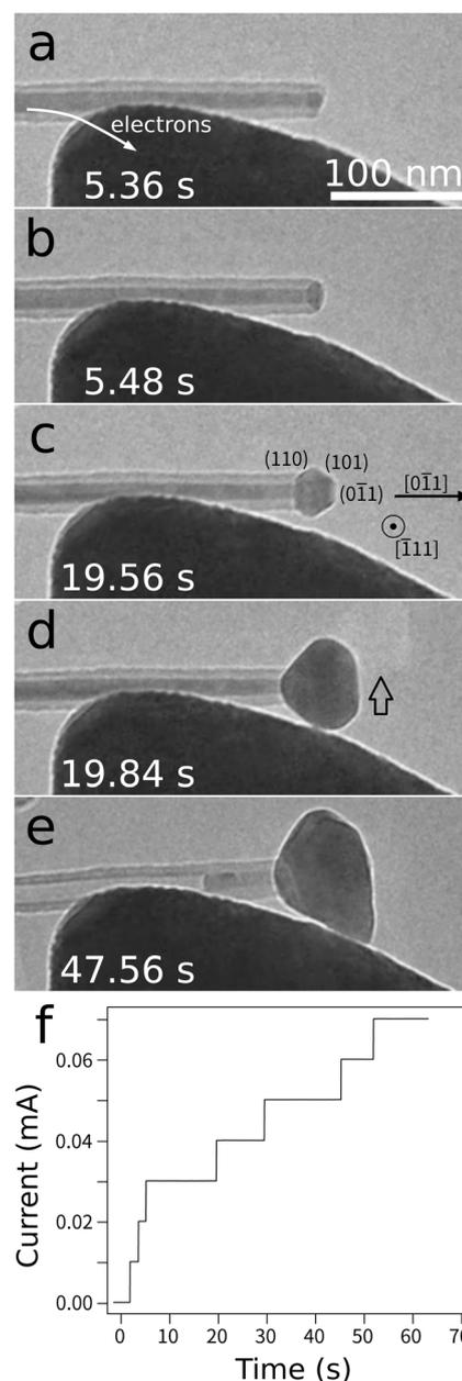
**Fig. 2** (a–e) *In situ* TEM images of electromigration manipulation of a Co nanorod filler. The Co filler was pushed out of the MWCNT to the right by the electromigration force. The arrow in (d) indicates a bright image of the portion of the Co nanorod outside the MWCNT formed with a Bragg-reflected wave. (f) Plot of current as a function of time (ESI movie† SM2 available).
