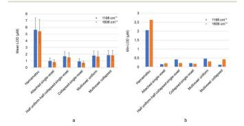
Fig. 8 The mean (a) and minimum (b) LOD over the measured map of the SERS substrates for BPE's peaks of interest in spectra averaged over each map. The bars, *i.e.* mean values, are calculated over multiple measured maps. The error bars show the map-to-map variation of the LOD.
