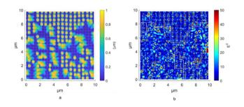
Fig. 5 AFM image (a) and FDTD simulation (b) of the single-voxelbased array with structures of 600 nm pitch, 490 nm diameter, and 850 nm height. Color bars represent (a) the height of the structures and (b) the electromagnetic field intensity.
