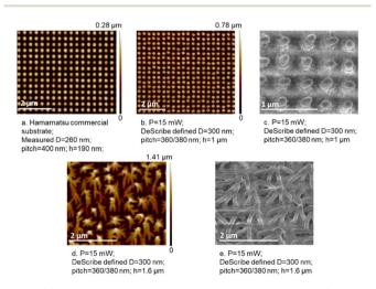
Fig. 4 (a) AFM image of Hamamatsu gold-coated dot array. (b and d) AFM and (c and e) SEM images of 2PP-fabricated nanostructures. The height of the structures is designed to be (b and c) 1 µm and (d and e) 1.6 µm. The pitch in XZ and YZ directions is respectively 360 and 380 nm, with a 300 nm voxel diameter.
