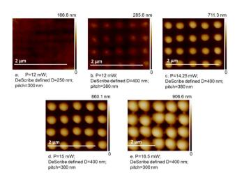
Fig. 3 AFM images of nanostructures fabricated with the multivoxelbased approach. (a and b) Correspond to the same lowest laser power with different height and pitch values. (c and d) Differ only in power values, and (e) corresponds to the highest applied laser power. Parameters here are the designed values given in Table 2 in ESI.†
