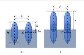
Fig. 1 Parameters of the voxel array. (a) Monolayer or so-called singlevoxel array; (b) accumulative or so-called multivoxel array.
