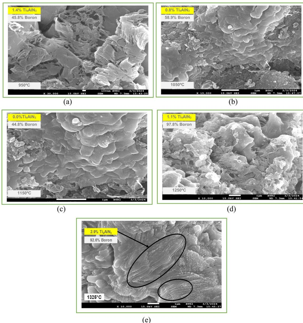
Fig. 8 FESEM images of the  $\text{Ti}_4\text{AlB}_2\text{N}$  composite (a) sample sintered at 950 °C, (b) sample sintered at 1050 °C, (c) sample sintered at 1150 °C, (d) sample sintered at 1250 °C and (e) sample sintered at 1325 °C.
