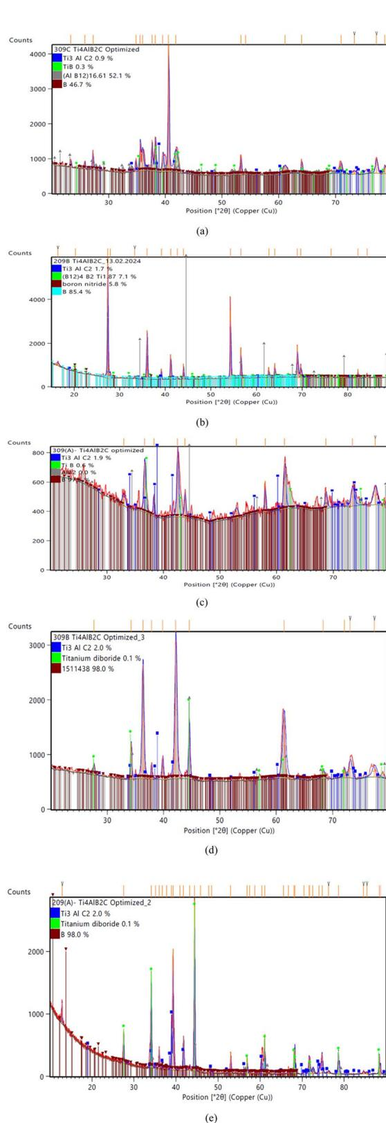
Fig. 5 Main graphics analysing the view of XRD patterns of  $\text{Ti}_4\text{AlB}_2\text{C}$  samples sintered at different temperatures: (a) sample sintered at 950 °C, (b) sample sintered at 1050 °C, (c) sample sintered at 1150 °C, (d) sample sintered at 1250 °C and (e) sample sintered at 1325 °C.
