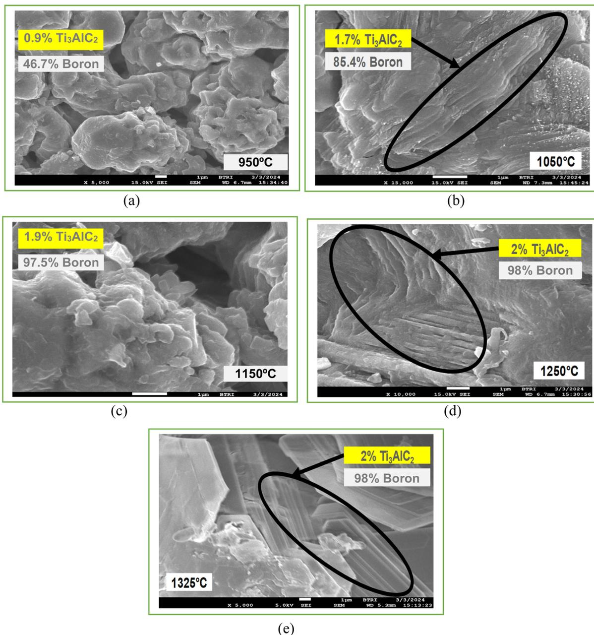
Fig. 9 FESEM images of the  $\text{Ti}_3\text{AlB}_2\text{C}$  composite (a) sample sintered at 950 °C, (b) sample sintered at 1050 °C, (c) sample sintered at 1150 °C, (d) sample sintered at 1250 °C and (e) sample sintered at 1325 °C.
