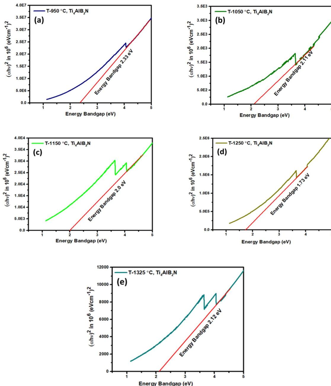
Fig. 14 Tauc plot for energy band gaps of  $\text{Ti}_4\text{AlB}_2\text{N}$  at different sintering temperatures: (a) sample sintered at 950 °C, (b) sample sintered at 1050 °C, (c) sample sintered at 1150 °C, (d) sample sintered at 1250 °C and (e) sample sintered at 1325 °C.
