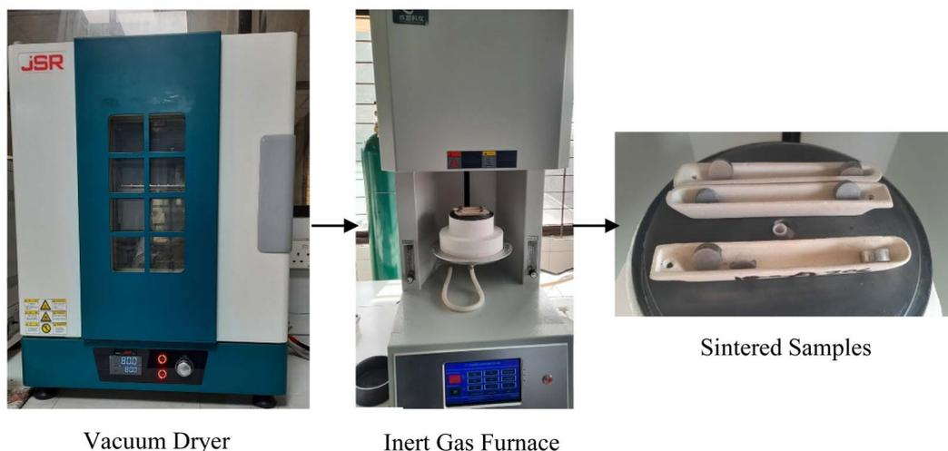
Fig. 2 Vacuum drying and inert gas sintering process.
