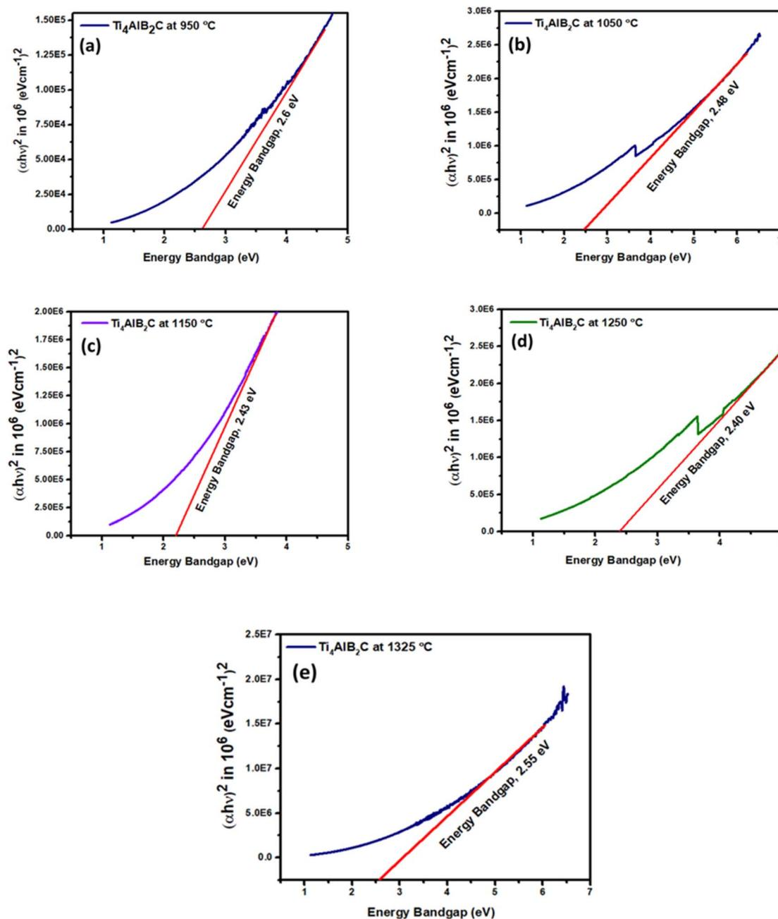
Fig. 15 Tauc plot for energy band gaps of  $\text{Ti}_4\text{AlB}_2\text{C}$  at different sintering temperatures: (a) sample sintered at 950 °C, (b) sample sintered at 1050 °C, (c) sample sintered at 1150 °C, (d) sample sintered at 1250 °C and (e) sample sintered at 1325 °C.
