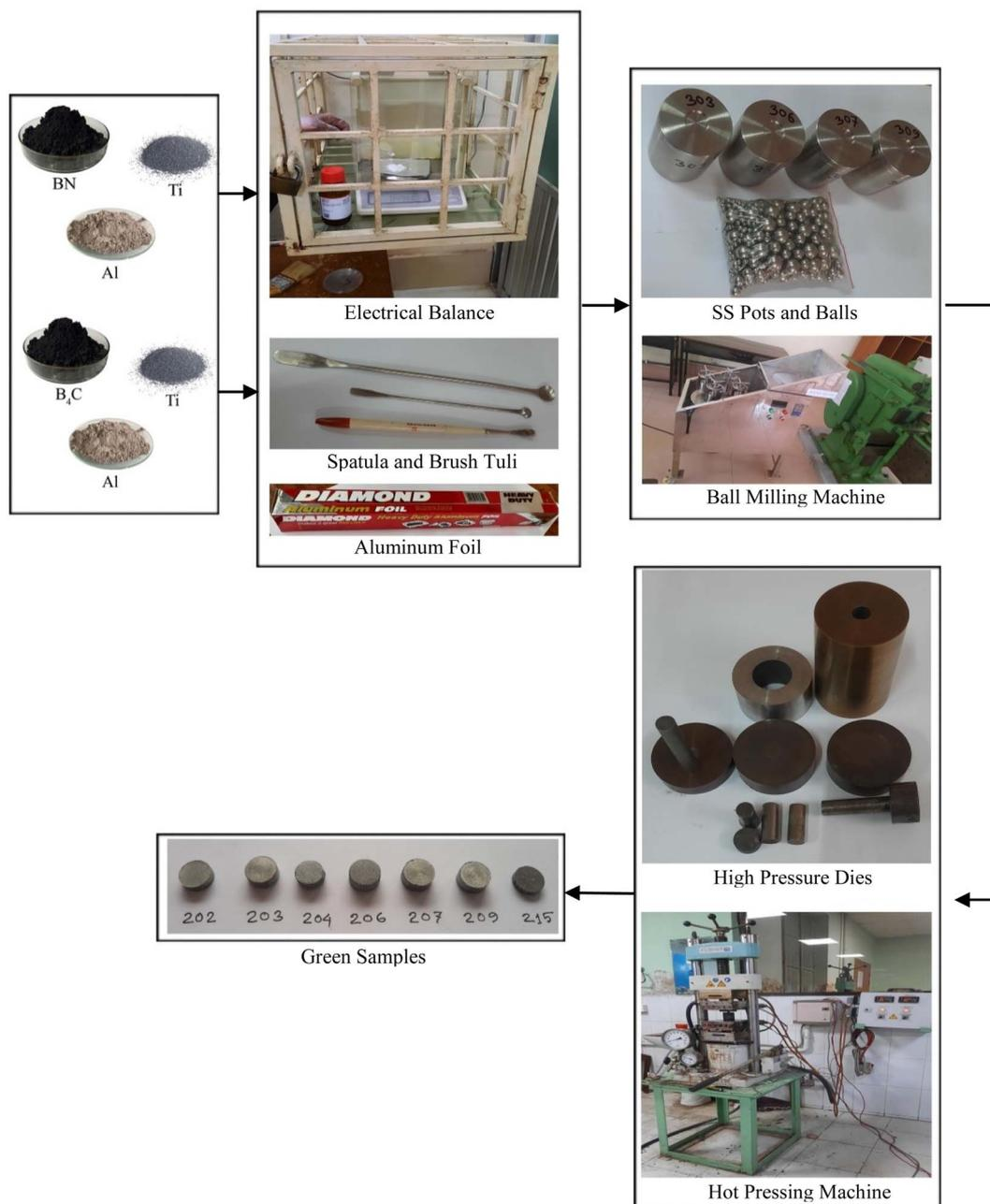
**Fig. 1** Synthesis process of green samples.
