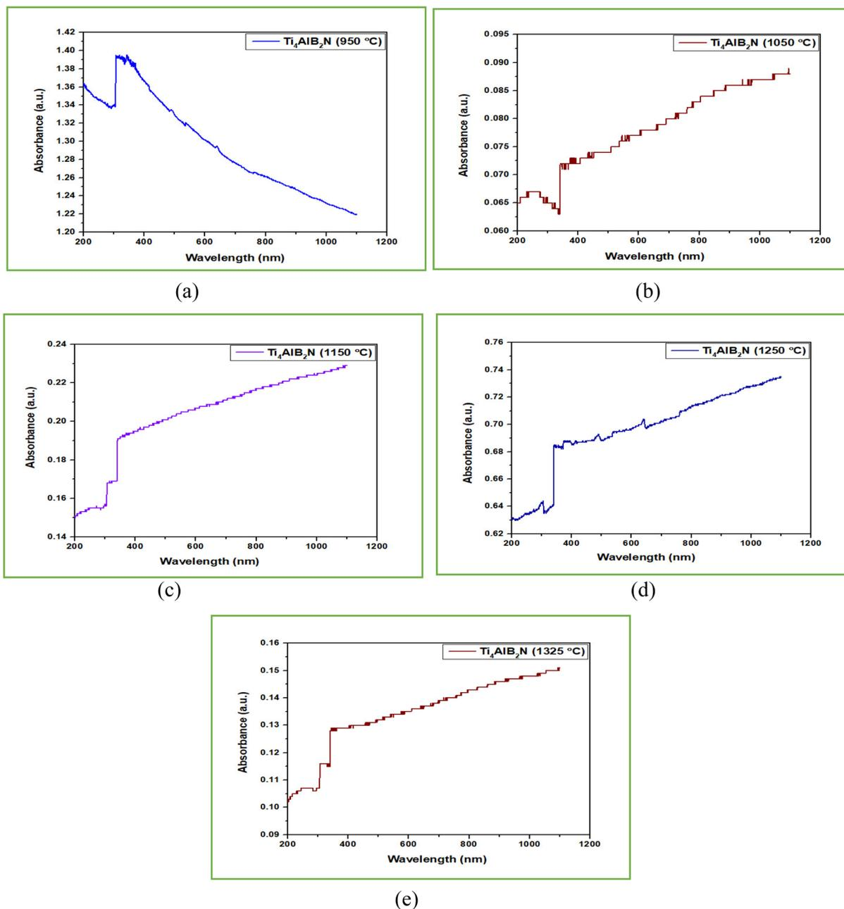
Fig. 12 UV analysis of  $\text{Ti}_4\text{AlB}_2\text{N}$  (absorbance vs. wavelength): (a) sample sintered at 950 °C, (b) sample sintered at 1050 °C, (c) sample sintered at 1150 °C, (d) sample sintered at 1250 °C and (e) sample sintered at 1325 °C.
