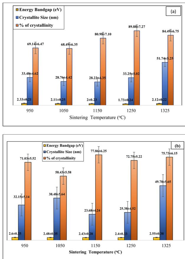
Fig. 7 Relation of % of crystallinity and crystallite size with energy bandgaps of fabricated boron based *in situ* MAX phase reinforced composites. (a)  $Ti_4AlB_2N$  (*in situ*  $Ti_4AlN_3$  MAX phase reinforced composite) and (b)  $Ti_4AlB_2C$  (*in situ*  $Ti_3AlC_2$  MAX phase reinforced composites).
