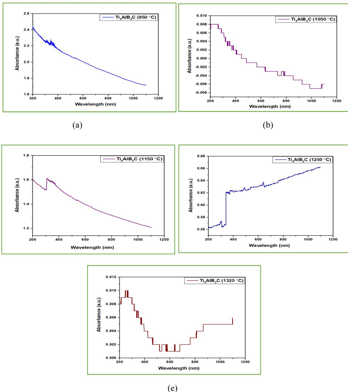
Fig. 13 UV analysis of  $\text{Ti}_4\text{AlB}_2\text{C}$  (absorbance vs. wavelength): (a) sample sintered at 950 °C, (b) sample sintered at 1050 °C, (c) sample sintered at 1150 °C, (d) sample sintered at 1250 °C and (e) sample sintered at 1325 °C.
