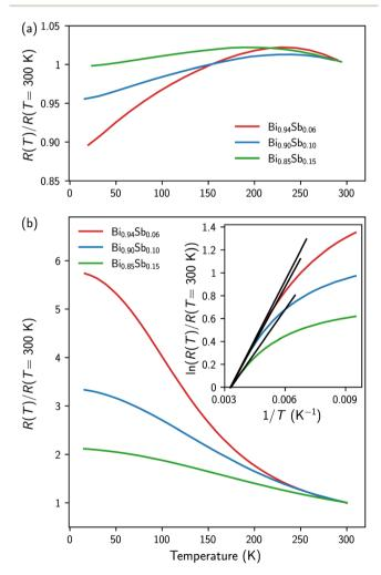
Fig. 3 (a and b) Temperature dependence of the electrical resistance of the as-prepared (a) and annealed (b)  $\mathrm{Bi}_{1-x}\mathrm{Sb}_x$  CNWs. The data are normalized to values obtained at room temperature. The inset of (b) shows the variation of the logarithm of the normalized resistance versus the inverse of temperature for the annealed samples.
