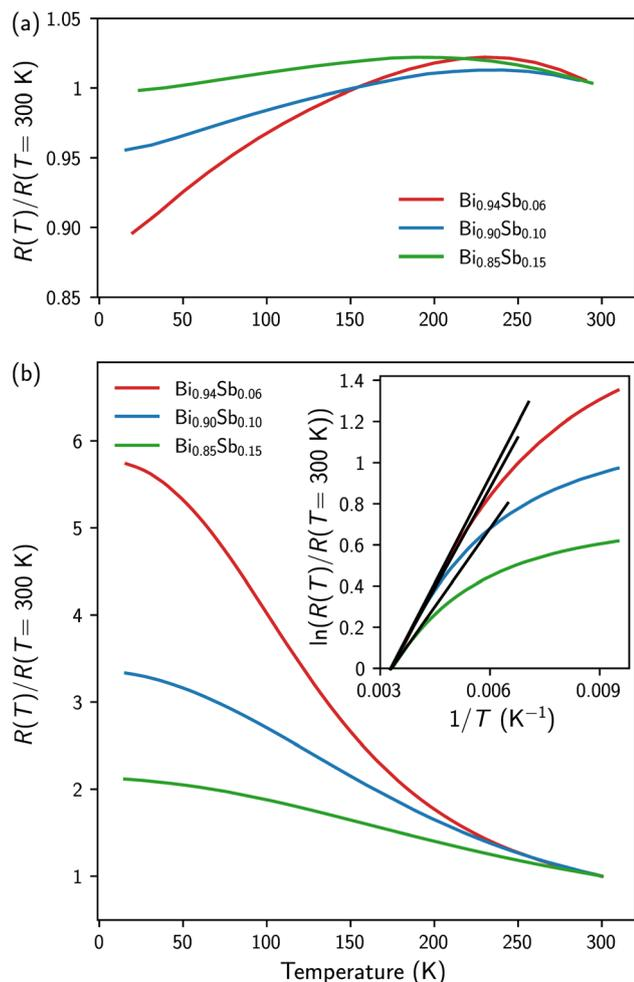
Fig. 3 (a and b) Temperature dependence of the electrical resistance of the as-prepared (a) and annealed (b)  $\text{Bi}_{1-x}\text{Sb}_x$  CNWs. The data are normalized to values obtained at room temperature. The inset of (b) shows the variation of the logarithm of the normalized resistance *versus* the inverse of temperature for the annealed samples.
