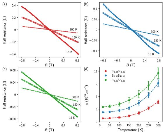
Fig. 4 (a-c) Magnetic field dependence of the Hall resistance of the annealed  $Bi_{1-x}Sb_x$  CNWs at different temperatures for x = 0.06 (a), x = 0.10(b) and x = 0.15 (c). (d) Temperature dependence of the carrier concentration of the annealed  $Bi_{1-x}Sb_x$  CNWs
