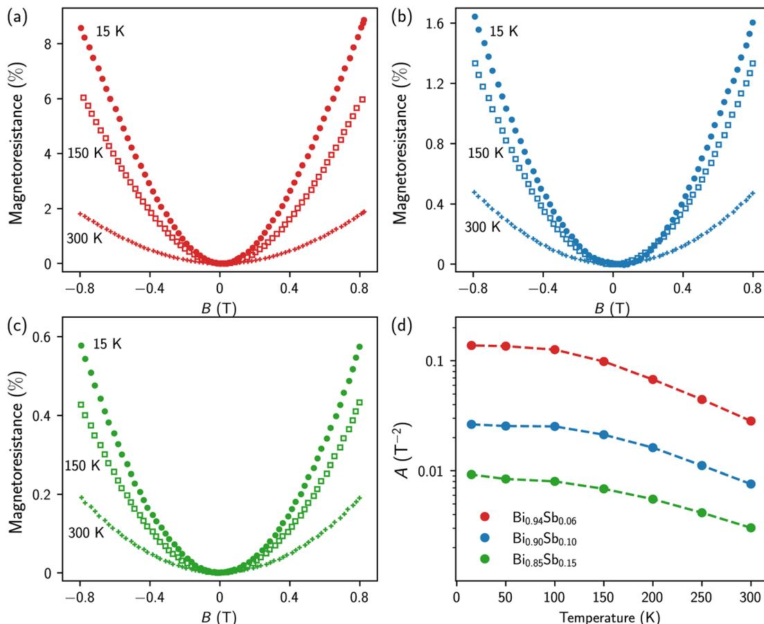
Fig. 5 (a–c) Magnetoresistance of annealed Bi<sub>1-x</sub>Sb<sub>x</sub> CNWs at different temperatures for  $x = 0.06$  (a),  $x = 0.10$  (b) and  $x = 0.15$  (c). (d) Temperature dependence of the amplitude of the magnetoresistance coefficient ( $A$ ), fitted in a range of  $\pm 0.8$  T.
