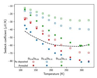
Fig. 6 Temperature dependence of the Seebeck coefficient of the asprepared and annealed  ${\rm Bi}_{1-x}{\rm Sb}_x$  CNWs. The dashed line shows the data obtained on a pure Bi CNW sample with the same diameter of 230 nm.<sup>14</sup>
