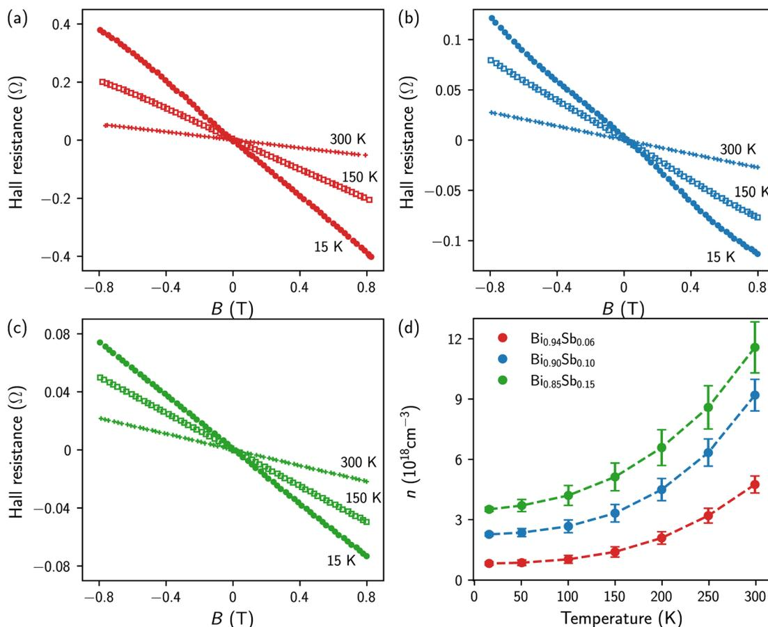
Fig. 4 (a–c) Magnetic field dependence of the Hall resistance of the annealed  $\text{Bi}_{1-x}\text{Sb}_x$  CNWs at different temperatures for  $x = 0.06$  (a),  $x = 0.10$  (b) and  $x = 0.15$  (c). (d) Temperature dependence of the carrier concentration of the annealed  $\text{Bi}_{1-x}\text{Sb}_x$  CNWs.
