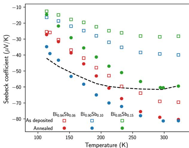
Fig. 6 Temperature dependence of the Seebeck coefficient of the as-prepared and annealed Bi<sub>1-x</sub>Sb<sub>x</sub> CNWs. The dashed line shows the data obtained on a pure Bi CNW sample with the same diameter of 230 nm.<sup>14</sup>
