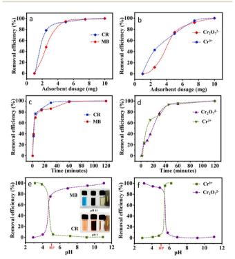
Fig. 3 The normalised removal efficiency of the cationic dye, MB, and the anionic dye, CR, with different (a) adsorbent dosage, (c) time and (e) pH. The normalised removal efficiency of  ${\rm Cr}^{3+}$  and  ${\rm Cr_2O_7}^{2-}$  with (b) adsorbent dosage, (d) time and (f) pH. The inset of (e) shows photographs of dye removal by NTA@SPIONs, followed by magnetic separation.
