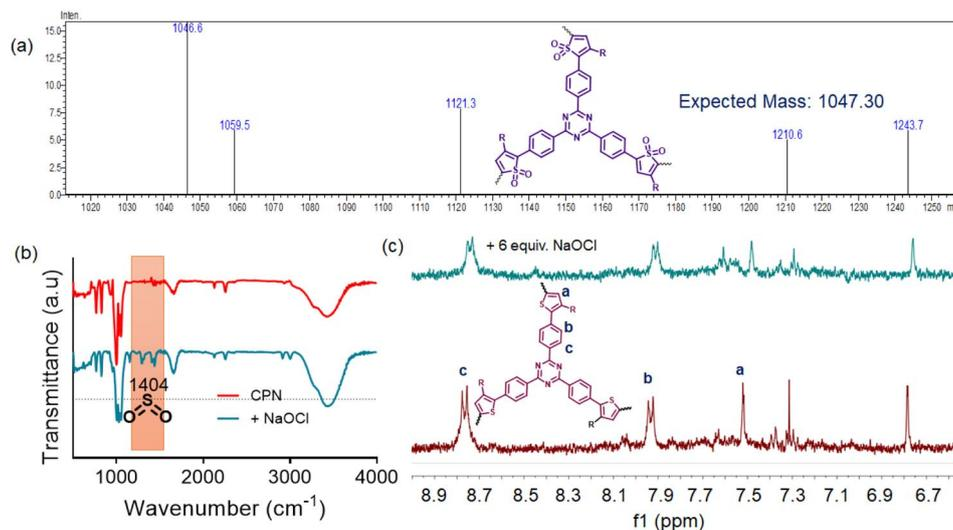
Fig. 7 (a) Mass spectra of probe CPN-NaOCl solution. (b) FTIR spectra of the CPN with and without the addition of NaOCl (6 equiv.). (c) Partial  $^1\text{H}$ -NMR of the CPN with and without hypochlorite NaOCl (6 equiv.) in  $\text{DMSO-}d_6$ .
