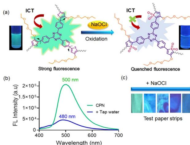
Fig. 8 (a) Plausible sensing mechanism of the CPN towards NaOCl. (b) Fluorescence spectra of the CPN ( $10\ \mu\text{M}$ ,  $\lambda_{\text{ex}} = 365\text{ nm}$ ) before and after exposure to tap water in THF : water (1 : 1) medium. (c) Images of the color change of pre-coated test paper strips upon exposure to increasing concentrations of hypochlorite (under UV light).
