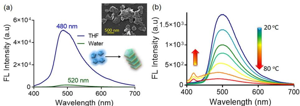
Fig. 3 (a) Fluorescence spectra of the CPN (10  $\mu\text{M}$ ,  $\lambda_{\text{ex}} = 365 \text{ nm}$ ) in THF and water and the FESEM image of the CPN in aqueous medium. (b) Temperature-dependent fluorescence spectra of the CPN (10  $\mu\text{M}$ ,  $\lambda_{\text{ex}} = 365 \text{ nm}$ ) in aqueous medium.
