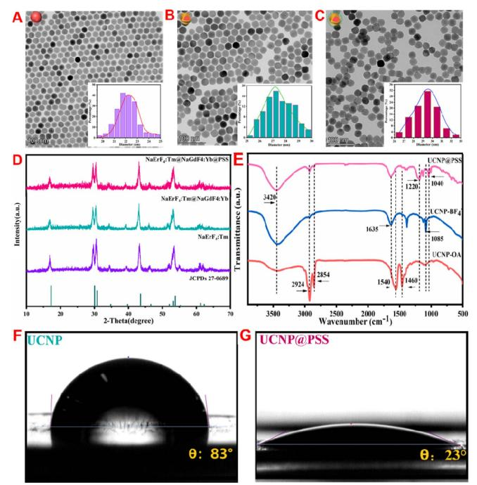
Fig. 2 (A-C) TEM, (D) XRD, (E) FT-IR, and (F and G) water contact angles of the prepared nanoparticles.
