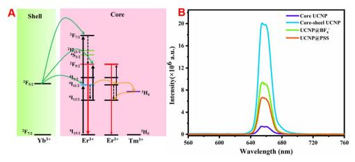
Fig. 3 (A) Schematic diagram of energy transfer inside the core-shell UCNPs (black solid arrows, orange arrows, green arrows and red solid arrows represent photon excitation, energy transfer, energy transfer and radiation emission, respectively) and (B) fluorescence spectra of the prepared nanoparticles.
