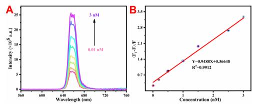
Fig. 7 (A) Fluorescence spectra of the system in the presence of various concentrations of miRNA-155 and (B) the correlation between the fluorescence recovery efficiency of the system and different concentrations of miRNA-155.
