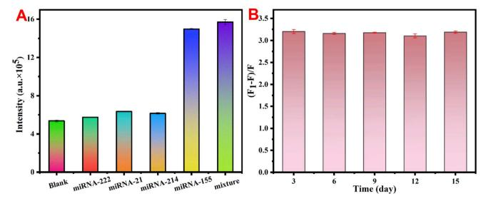
(A) Effects of different miRNAs on the fluorescence intensity and (B) stability of the detection system
