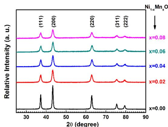
Fig. 1 XRD pattern analysis of pure NiO and Mn-doped NiO NPs.
