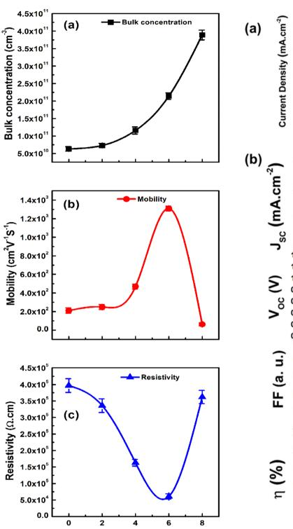
Fig. 7 (a) Bulk concentration variation of the bulk NiO NPs thin films, (b) mobility of free carriers in the NiO NPs thin films, and (c) resistivity of the NiO NPs thin films variation with Mn doping percentage.
