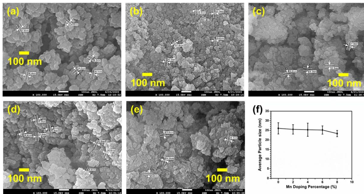
Fig. 2 FE-SEM morphological images of the synthesized  $\text{Ni}_{1-x}\text{Mn}_x\text{O}$  NPs:  $x =$  (a) 0, (b) 0.02, (c) 0.04, (d) 0.06, (e) 0.08 and variation of average particle size of NiO NPs with Mn doping percentage (f).
