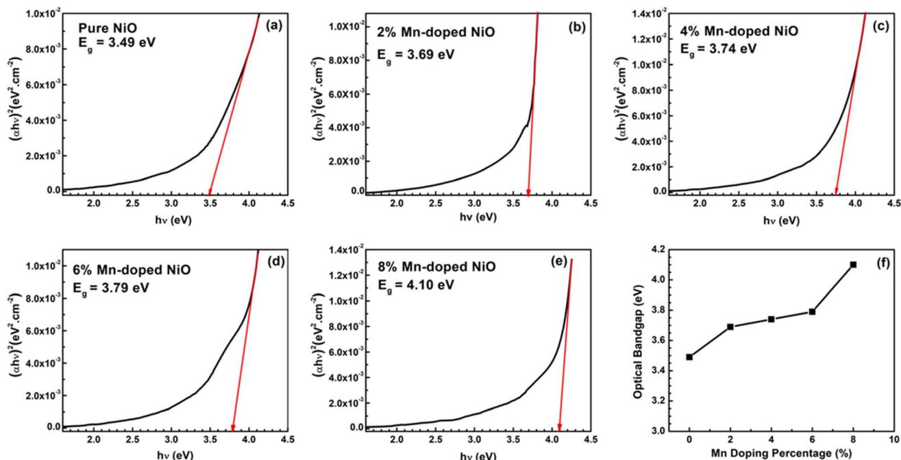
Fig. 6 Tauc plot of the  $\text{Ni}_{1-x}\text{Mn}_x\text{O}$  NPs: (a)  $x = 0$ , (b)  $x = 0.02$ , (c)  $x = 0.04$ , (d)  $x = 0.06$ , (e)  $x = 0.08$ . And variation of NiO NPs optical bandgap with different Mn doping concentrations (f).
