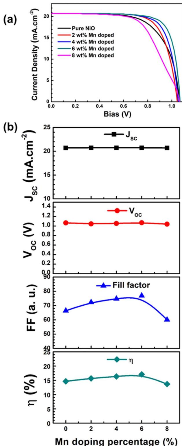
Fig. 8 (a)  $J$ - $V$  curve of SCAPS-1D simulated Perovskite based solar cells using synthesized pure and Mn-doped NiO NPs thin film based HTL layer and (b) device performance parameter variation of different devices.
