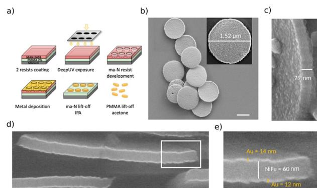
Fig. 1 (a) Nanofabrication process of the vortex microdiscs. (b and c) SEM images after particle release from the wafer showing top (b) and side (c) views of the NPs. Scale bar: 1  $\mu\text{m}$ . (d) View of the lateral cross-section of particles, obtained with FIB-SEM. (e) Zoom of the region enclosed in the white rectangle in (d).
