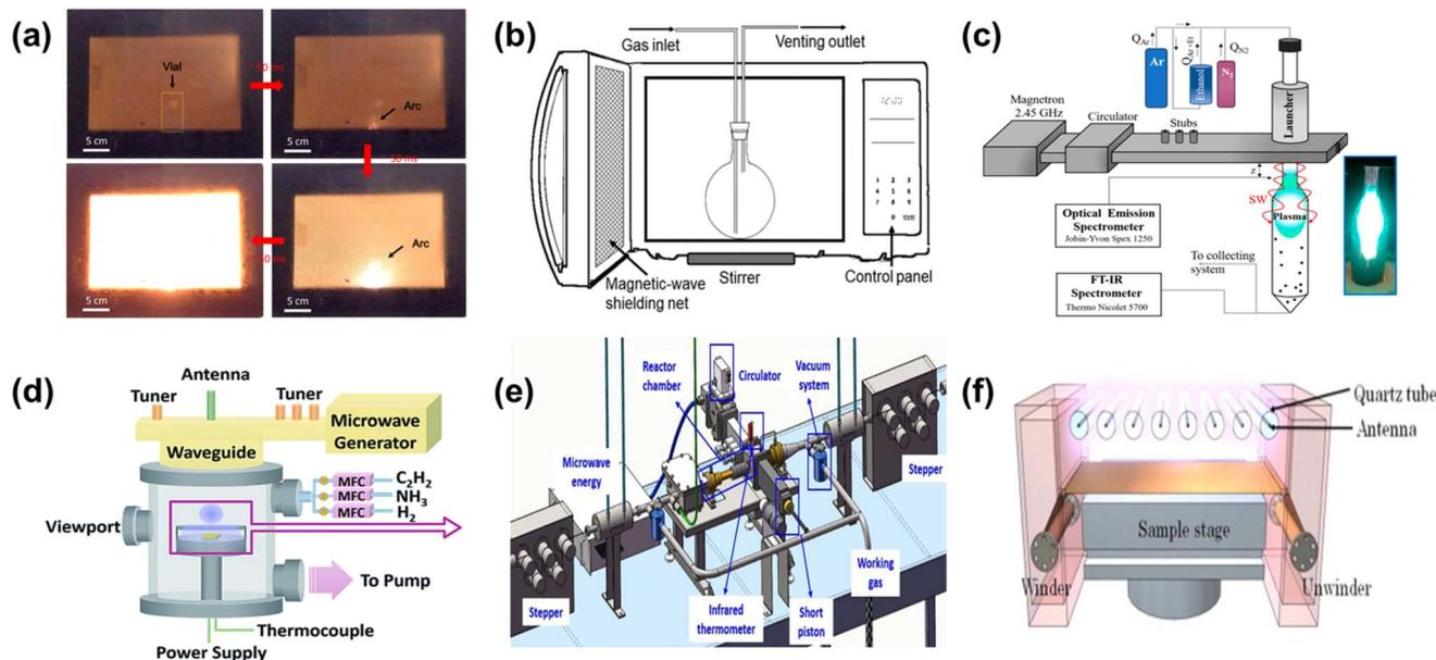
Fig. 4 Schematic diagram of various types of microwave reactors. (a) The domestic microwave oven. (b) Adapted domestic microwave oven. (c) Typical composition diagram of a MPCVD reactor. (d) MPCVD for large area reaction zone type. (e) Continuous microwave plasma reactor systems for the production of fibres. (f) Systems of a roll-to-roll microwave plasma reactor.
