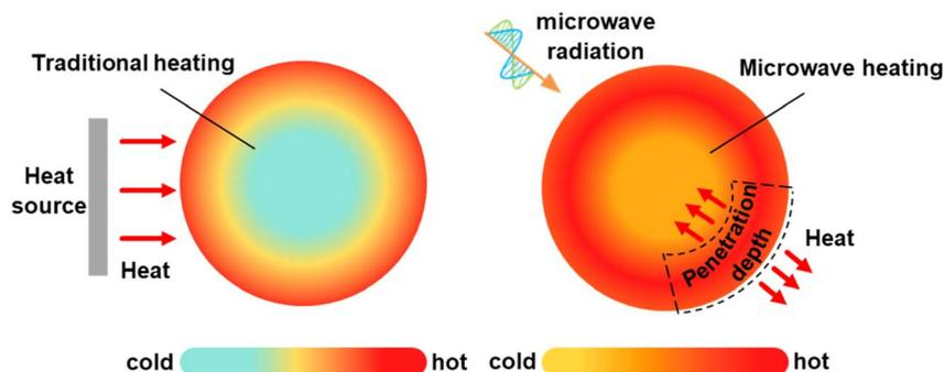
Fig. 3 Different heating models for conventional and microwave heating.
