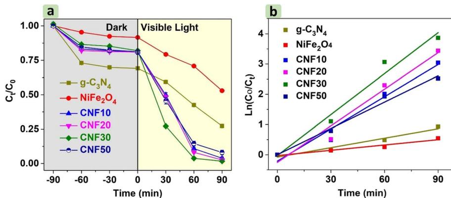
Fig. 7 Photocatalytic degradation of RhB by  $g\text{-C}_3\text{N}_4$ ,  $\text{NiFe}_2\text{O}_4$ , and  $\text{CNF}_x$  ( $x = 10, 20, 30, 50$ ) (a), and photodegradation kinetics fitted by the pseudo-first-order model (b).
