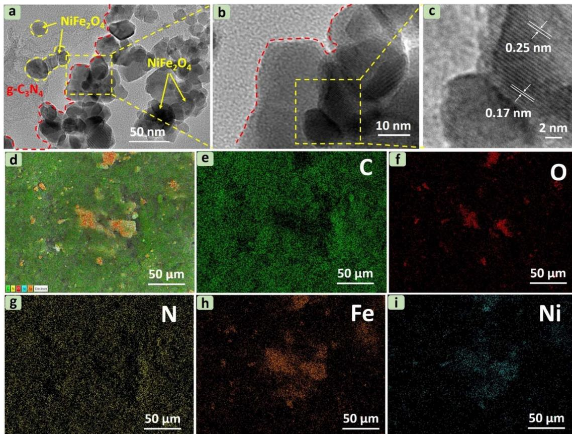
Fig. 4 HR-TEM (a–c) and EDS mapping (d–i) of CNF30.
