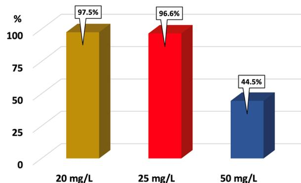
Fig. 10 The effect of RhB initial concentration on the photodegradation efficiency of CNF30 (H<sub>2</sub>O<sub>2</sub>: 0.2 M, dose: 1.5 g L<sup>-1</sup>).
