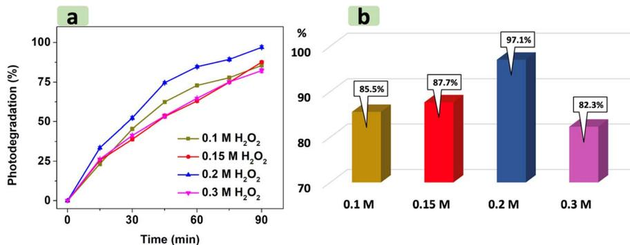
Fig. 9 Effect of H<sub>2</sub>O<sub>2</sub> concentration on RhB photocatalytic degradation under visible light (a), the RhB degradation percentage after 90 min at various H<sub>2</sub>O<sub>2</sub> concentrations (b).
