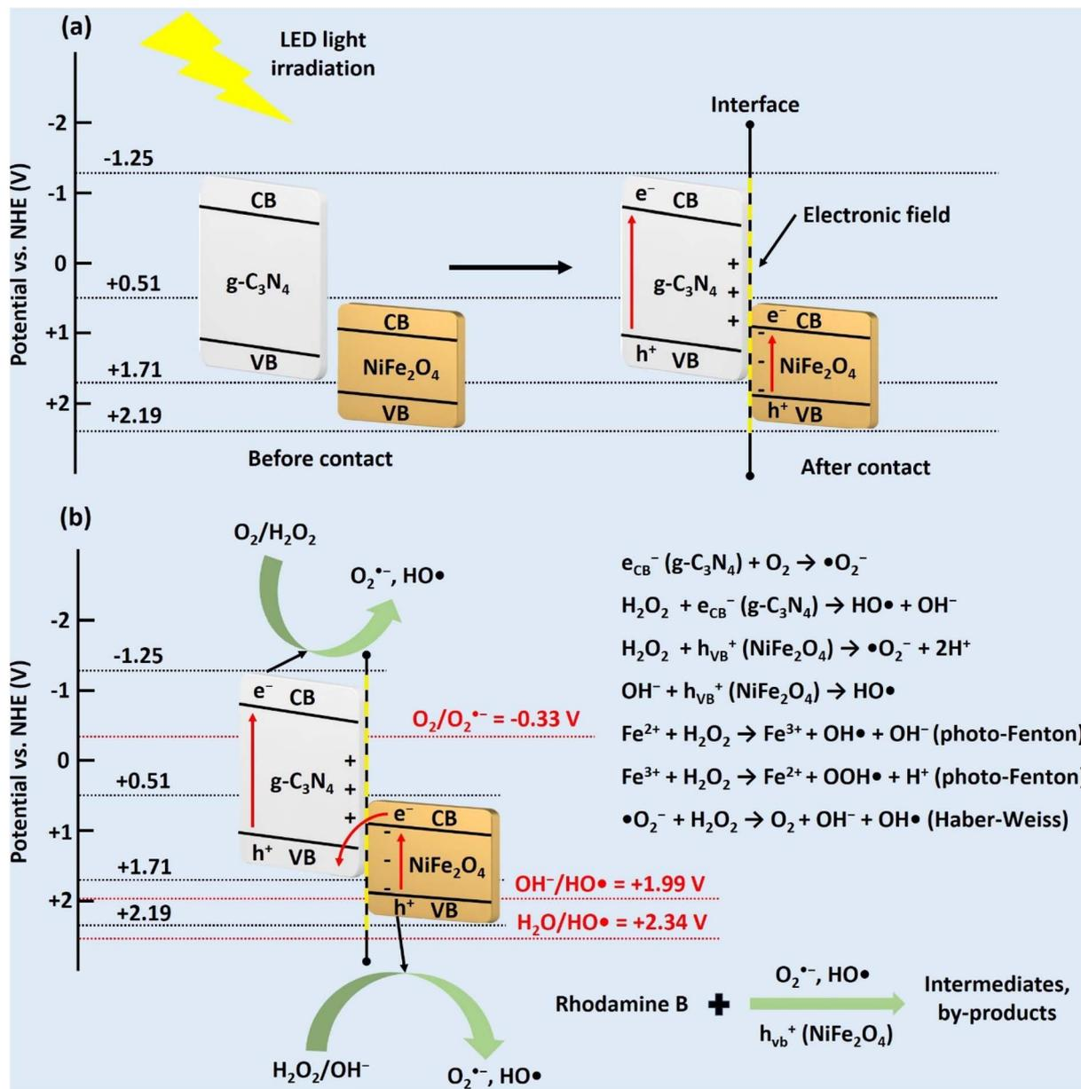
Fig. 12 Proposed mechanism of RhB photodegradation by NiFe<sub>2</sub>O<sub>4</sub>/g-C<sub>3</sub>N<sub>4</sub>. After receiving photon energy, electric fields, coulombic repulsion, and band bending, which hinder type-II heterojunction and support the S-scheme mechanism (a). The RhB photodegradation process involves radical species (b).
