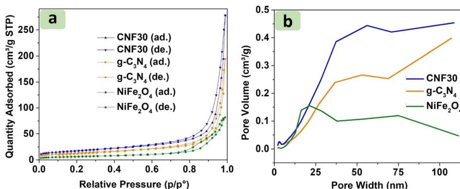
Fig. 5  $\text{N}_2$  adsorption–desorption isotherm curves (a) and BJH adsorption  $dV/d \log(w)$  pore volume (b) of  $g\text{-C}_3\text{N}_4$ ,  $\text{NiFe}_2\text{O}_4$ , and CNF30.
