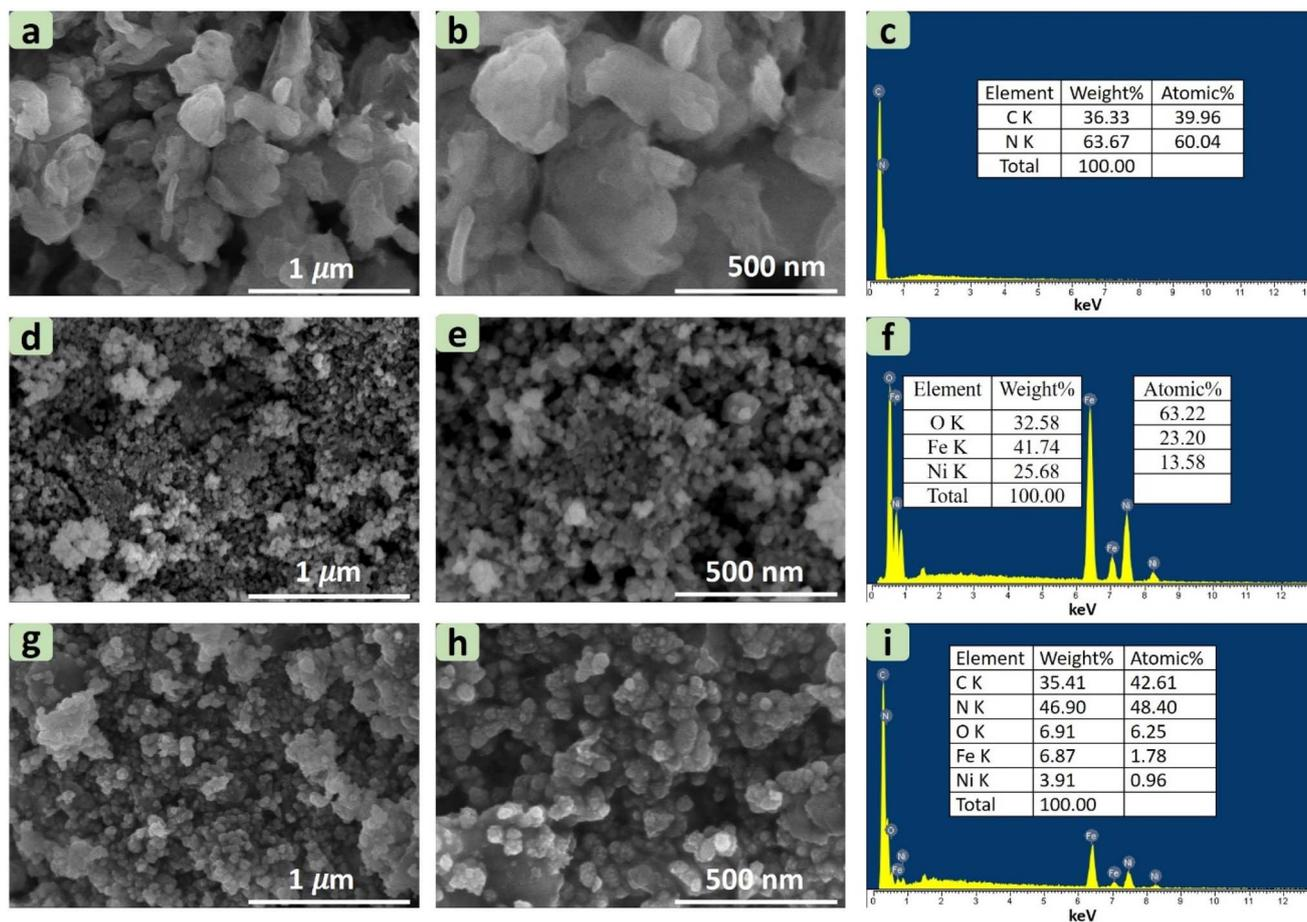
Fig. 3 SEM images of g-C<sub>3</sub>N<sub>4</sub> (a and b) and EDX analysis (c). SEM images of NiFe<sub>2</sub>O<sub>4</sub> (d and e) and EDX analysis (f). SEM images of CNF30 (g and h) and EDX analysis (i).
