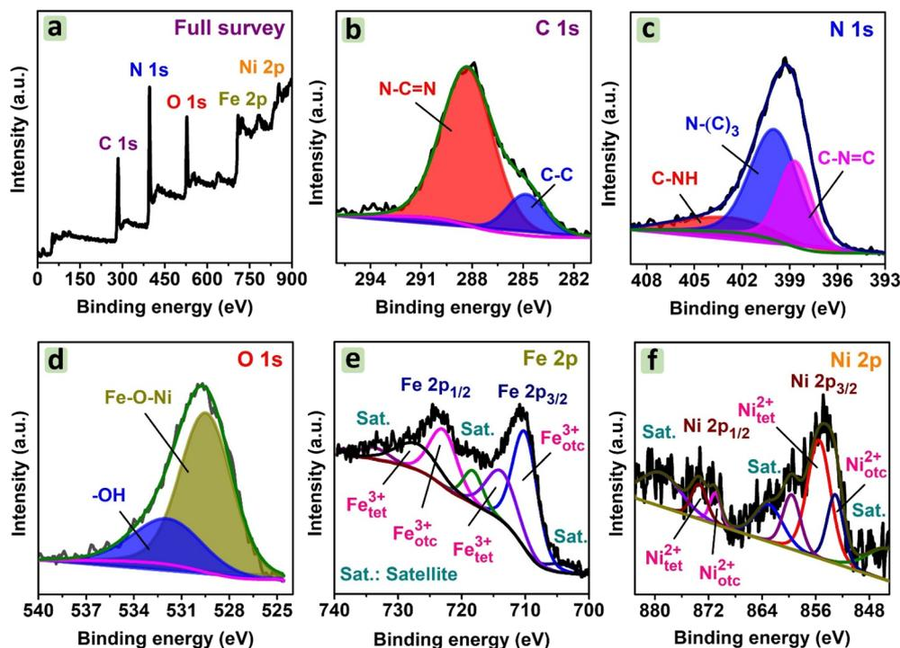
Fig. 6 XPS analysis of CNF30: (a) full survey, (b) C1s, (c), N1s, (d) O1s, (e) Fe 2p, and (f) Ni 2p.
