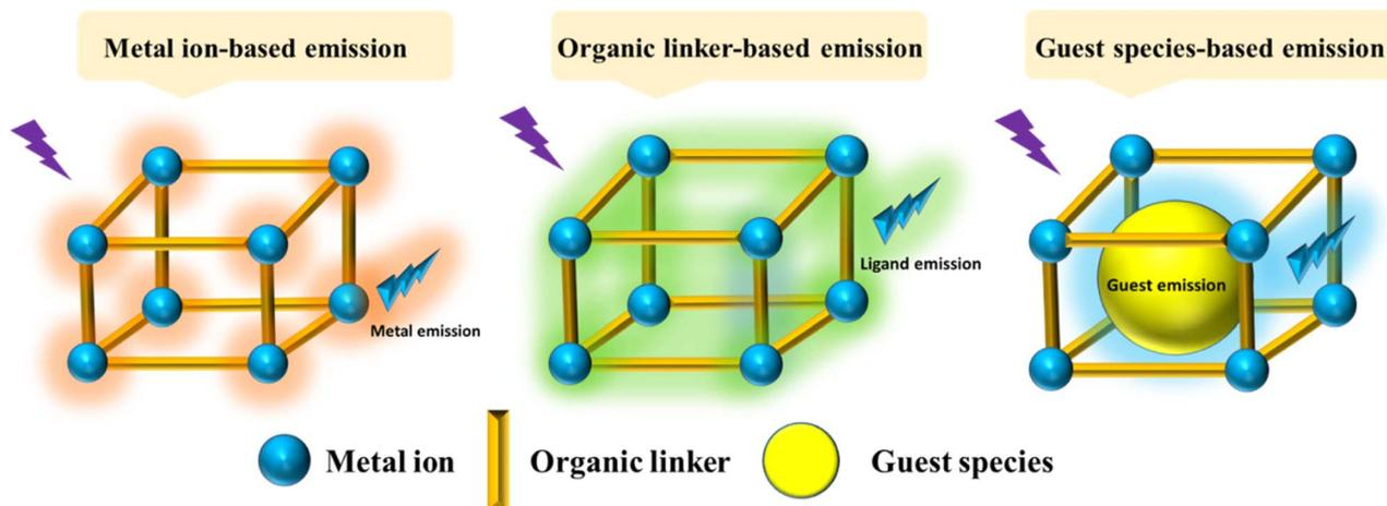
Fig. 2 Illustration of potential emission modes in MOFs.
