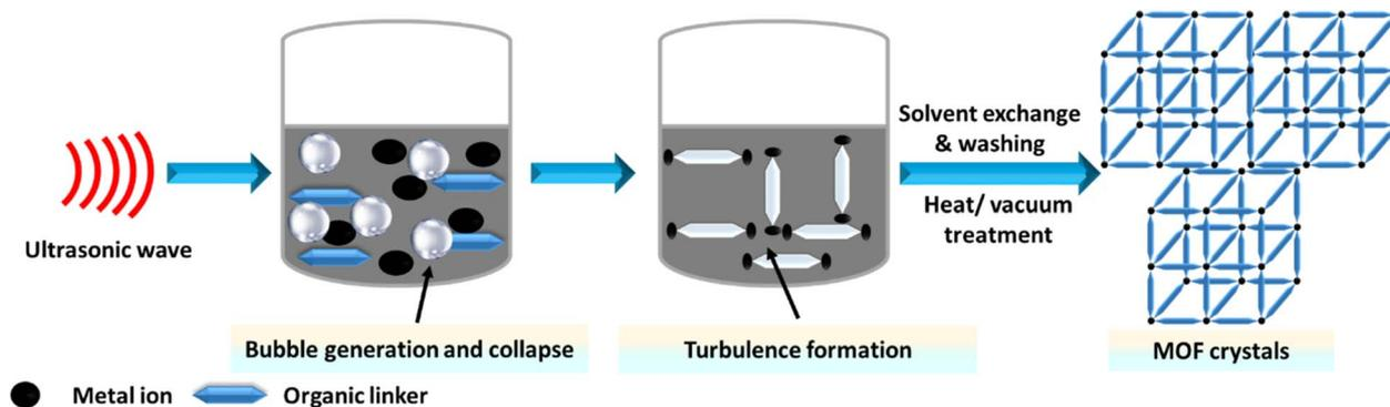
Fig. 8 Sonochemical synthesis of MOF structures.
