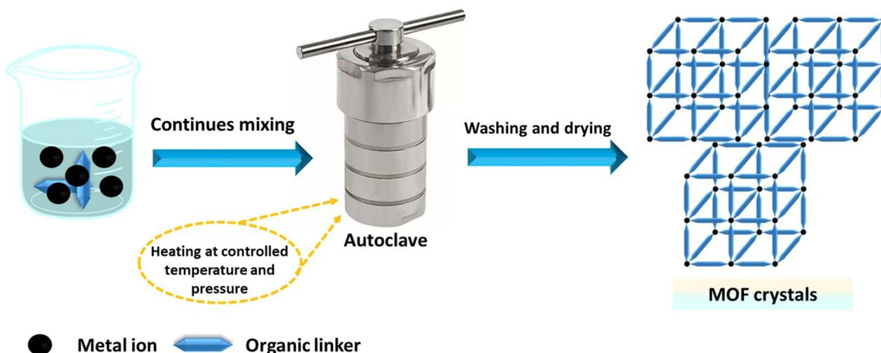
Fig. 6 Schematic representation of the hydrothermal/solvothermal synthesis route.
