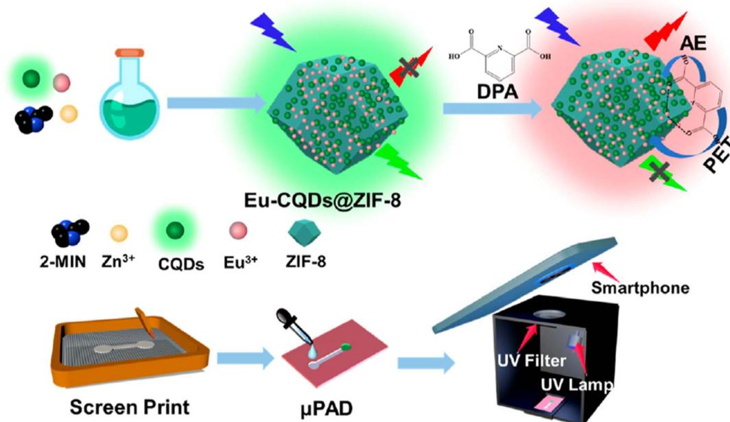
Fig. 23 Schematic depiction of the preparation process for (A)  $\text{Eu-CQDs@ZIF-8}$  and (B)  $\mu\text{PAD}$  used in DPA detection. Adapted from ref. 278 with permission. Copyright 2024, American Chemical Society.
