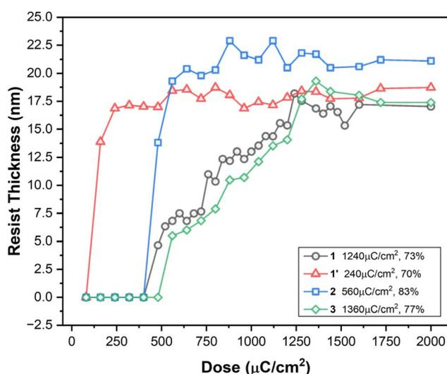
Fig. 5 Contrast curves of the four clusters using e-beam sources; initial thickness is 25 nm, 24 nm, 27.0 nm, and 25.0 nm for clusters (1), (1'), (2), and (3) respectively. Cluster (1') refers to  $(\text{vinylSn})_6(\text{sec-C}_4\text{H}_9\text{CO}_2)_8\text{O}_4\text{Cl}_2$ .<sup>9</sup> The developers are acetone (10 s) for cluster (2) and 2-heptanone (60 s) for cluster (3).
