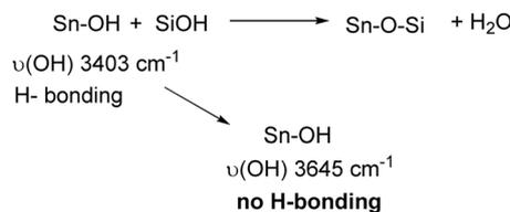
Scheme 2 Proposed chemical reactions with EUV exposure.
