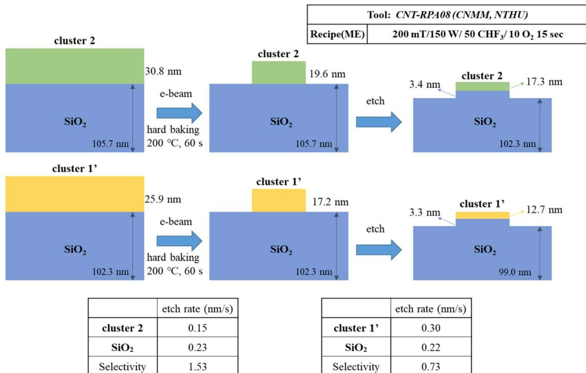
Fig. 13 Comparison of etching resistance between clusters (1') and (2).
