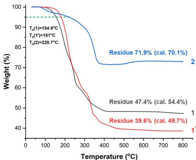
Fig. 1 Thermal gravimetric analysis of clusters (1), (1'), and (2); cluster (1') refers to  $(\text{vinylSn})_6(\text{sec-C}_4\text{H}_9\text{CO}_2)_8\text{O}_4\text{Cl}_2$ .<sup>9</sup>
