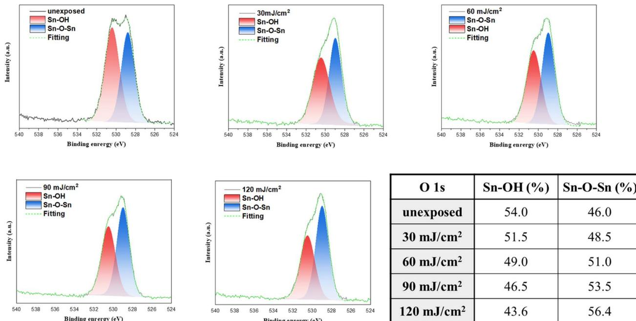
Fig. 12 Band shape fitting of the O(1s) component of cluster (2) at different EUV doses.
