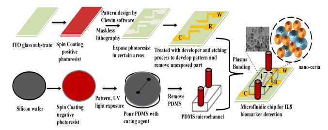
Scheme 1 Steps for the preparation of a microfluidic chip using the maskless lithography technique
