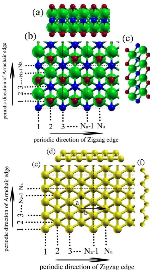
Fig. 1 (a), (c), (d) and (f) side views and (b) and (e) top views of  $M_2XT_2$  nanoribbons and striped borophene nanoribbons, respectively. M, X, T, and B elements are depicted in green, blue, red, and gold colors, respectively.
