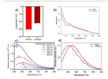
Fig. 2 (a) Z-potential values of RCDs and L-RCDs; (b) absorption spectra of RCDs (0.102 mg mL<sup>-1</sup>) and L-RCDs (1.056 mg mL<sup>-1</sup>) in room-temperature water solutions; (c) emission spectra of L-RCDs in H<sub>2</sub>O at 298 K upon excitation in the range of 500-600 nm; (d) normalized emission spectra of RCDs and L-RCDs in  $H_2O$  ( $\lambda_{ex}$  540 nm).
