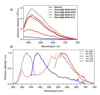
Fig. 5 (a) Screening of the emission of Resin-R containing increasing amounts of L-RCDs ( $\lambda_{exc} = 500$  nm); (b) normalized excitation (dashed) and emission (solid) spectra of printed Resin-R@L-RCDs-0.2% at different wavelengths.
