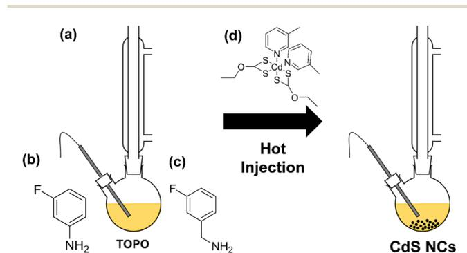
Fig. 1 (a) Reaction scheme of the hot injection method to form colloidal CdS nanocrystals. Also shown are the chemical structures of (b) 3-FLAn, (c) 3-FLBzAm and (d) [Cd(Xan)<sub>2</sub>(3mpy)<sub>2</sub>].
