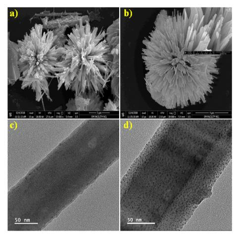
Fig. 3 FESEM images: (a) low magnification  $Bi_2S_3$  microflowers, (b) high magnification  $Bi_2S_3$  with the inset displaying nanorods; TEM images (c and d) of bare Bi<sub>2</sub>S<sub>3</sub> and Au decorated Bi<sub>2</sub>S<sub>3</sub> NRs, respectively.
