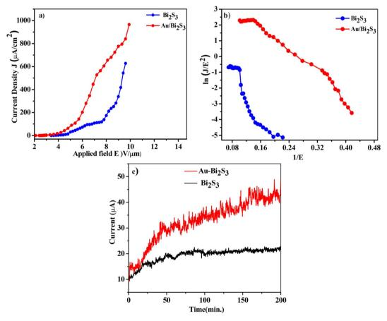
Fig. 6 Plot of field emission current density versus applied electric field (J-E) (a), Fowler-Northeim (F-N) plot (b) of  $Bi_2S_3$  and  $Au/Bi_2S_3$ , respectively. (c) Field emission current stability plots at 10  $\mu$ A.
