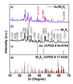
Fig. 2 XRD of the (a) Au/Bi<sub>2</sub>S<sub>3</sub> sample and (b) Bi<sub>2</sub>S<sub>3</sub>; (c) and (d) are JCPDS cards of Au and Bi<sub>2</sub>S<sub>3</sub> crystals, respectively.
