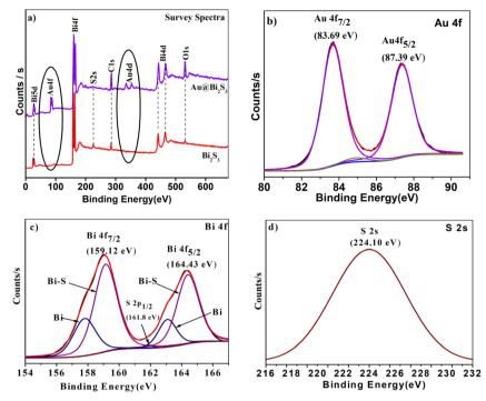
Fig. 5 XPS images of (a)  $Bi_2S_3$  and  $Au/Bi_2S_3$  survey spectra; high resolution spectra of (b)  $Au^0$  state, (c)  $Bi^{3+}$  state, (d)  $S^{2-}$  state of the  $Au/Bi_2S_3$ sample.
