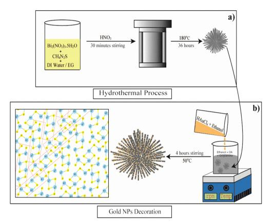
Fig. 1 Schematic depiction of the mechanism of (a) the hydrothermal synthesis of Bi<sub>2</sub>S<sub>3</sub> microflowers, (b) Au decoration process on assynthesized Bi<sub>2</sub>S<sub>3</sub> NRs and schematic structure of Bi<sub>2</sub>S<sub>3</sub>
