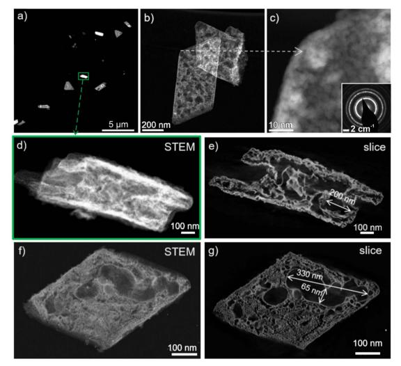
Fig. 4 Electron microscopy and tomography of CeO2 nanosponges: (a-d and f) HAADF-STEM images at different magnification (inset in (c) showing the crystallinity, ESI Fig. S4†), (e and g) examples of Z-slices obtained from 3D electron tomographic reconstructions of nanosponges shown in (d) and (f) (for volume rendering and reconstruction of Z-slices see ESI Fig. S5 and Videos S1-S4†).
