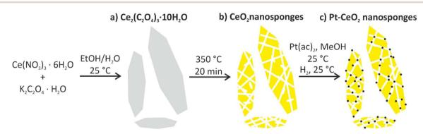
Fig. 1 Scheme illustrating the synthesis of Pt–CeO<sub>2</sub> nanosponges: (a) formation of rod- to platelet-shaped  $Ce_2(C_2O_4)_3 \cdot 10H_2O$  precursor particles, (b) thermal conversion of  $Ce_2(C_2O_4)_3 \cdot 10H_2O$  precursor particles to  $CeO_2$  nanosponges, (c) wet-chemical impregnation of the  $CeO_2$  nanosponges with a solution of  $Pt(ac)_2$  in methanol followed by Pt nanoparticle formation (at 25 °C).
