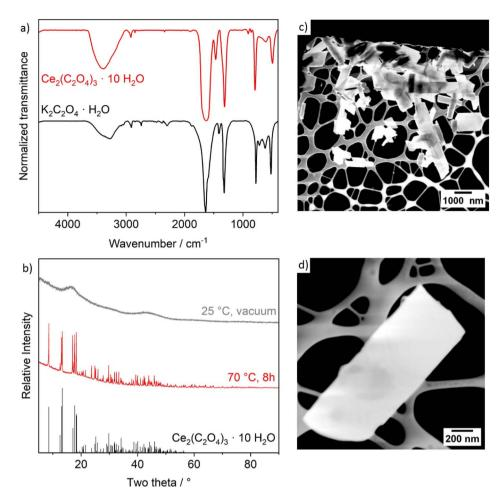
Fig. 2 Characterization of the  $Ce_2(C_2O_4)_3 \cdot 10H_2O$  precursor particles: (a) FT-IR spectrum  $(K_2C_2O_4 \cdot H_2O)$  as a reference), (b) XRD  $(Ce_2(C_2O_4)_3 \cdot H_2O)$ ·10H<sub>2</sub>O as a reference, ICDD-No. C01-075-7101), (c) STEM overview image, (d) STEM detail image of a single precursor particle.
