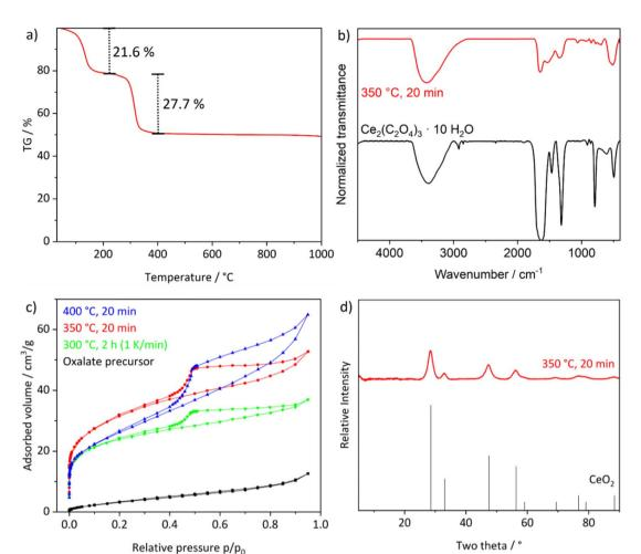
Fig. 3 Characterization of the  $CeO_2$  nanosponges: (a) thermogravimetric analysis, (b) FT-IR spectra before and after thermal conversion, (c) volumetric sorption analysis after different thermal treatments, (d) XRD ( $CeO_2$  as a reference, ICDD-No. C00-034-0394).
