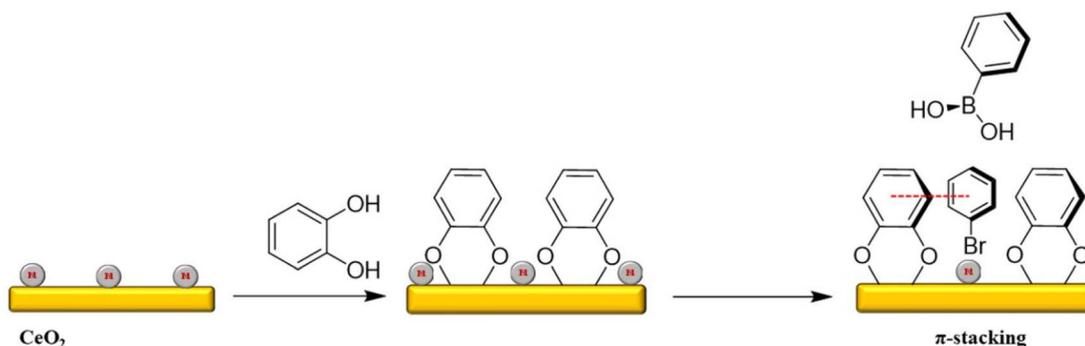
Fig. 22 A schematic representation of CTE modification of Pd/CeO<sub>2</sub> and subsequent  $\pi$ -stacking between CTE and substrates.
