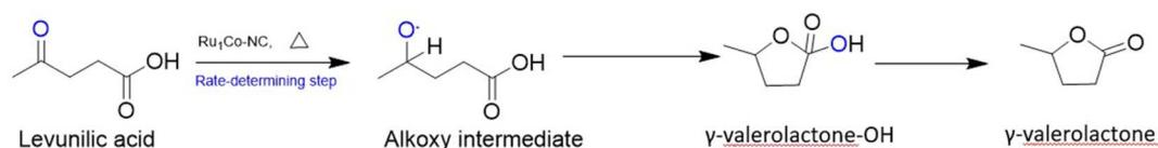
Fig. 14 Schematic of levulinic acid conversion into  $\gamma$ -valerolactone catalyzed by Ru<sub>1</sub>Co-NC SAC.
