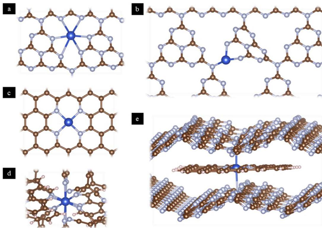
Fig. 24 An illustration of the structural features of Cu adsorbed in the heptazine pore of mpgC<sub>3</sub>N<sub>4</sub> (a) C substituted by Cu in mpgC<sub>3</sub>N<sub>4</sub> (b) dicarbon vacancy in N-doped graphene hosted by Cu (c), octahedral complex [Cu(bpy)(tcm)<sub>4</sub>]<sup>2+</sup> (d) and sandwich-like arrangement of Cu-doped N-graphene intercalated in mpgC<sub>3</sub>N<sub>4</sub> (e). Reproduced with permission from ref. 179. Copyright 2022, ACS Catal.
