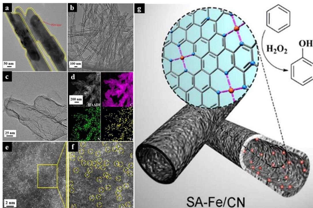
Fig. 16 TEM images of (a)  $\alpha$ -FeOOH@PDA; (b and c) SA-Fe/CN. (d) HAADF-STEM image and corresponding EDX mapping of SA-Fe/CN, C (pink), N (green) and Fe (yellow). (e and f) AC HAADF-STEM image and enlarged view of SA-Fe/CN. (g) An illustration of core-shell structured SA-M/CN materials for direct hydroxylation of benzene to phenol. Reproduced with permission from ref. 130. Copyright 2017, *J. Am. Chem. Soc.*
