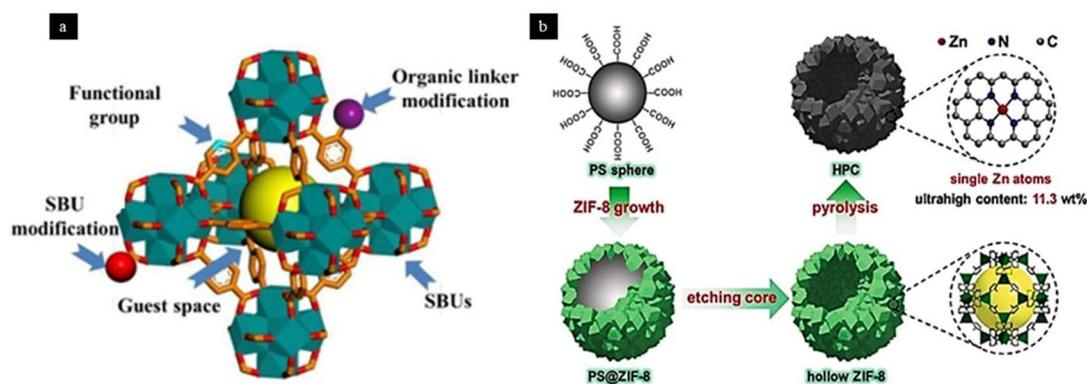
Fig. 8 A depiction of (a) different anchoring sites of an MOF. Reproduced with permission from ref. 56. Copyright 2020, *Energy Environ. Sci.* (b) Hollow porous carbon supported Zn SAC prepared from an MOF precursor. Reproduced with permission from ref. 59. Copyright 2019, *Angew. Chem. Int. Ed.*
