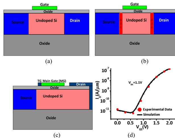
Fig. 1 Schematics of (a) conventional SBMOSFET, (b) DSL SBMOSFET and (c) proposed GDE-SBMOSFET. (d) Model Calibration using experimental data.<sup>19</sup>
