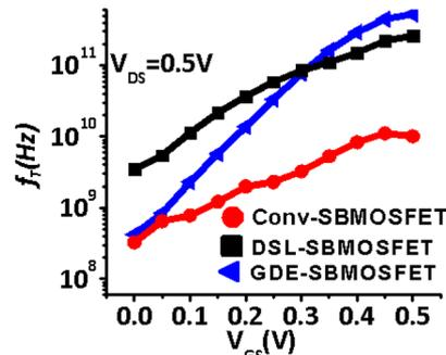
Fig. 9 Cutoff frequency ( $f_T$ ) comparison of all three devices.
