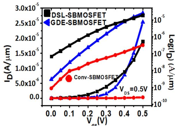
Fig. 5 Transfer characteristics of GDE-SBMOSFET, DSL-SBMOSFET and conventional SBMOSFET.
