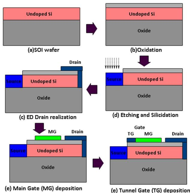
Fig. 2 Process flow of the proposed device.
