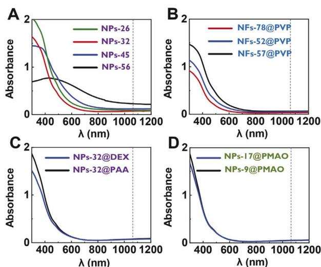
Fig. 2 UV-Vis-NIR spectra at  $0.1 \text{ mg}_{\text{Fe}} \text{ mL}^{-1}$  in the range of 300–1200 nm of (A) uncoated octahedral nanoparticles with sizes between 26 and 56 nm, (B) nanoflowers with the same core size (8–10 nm) and coating (polyvinylpyrrolidone) and different particle sizes (52–78 nm), (C) 32 nm octahedral nanoparticles with different coatings, and (D) spherical nanoparticles with sizes of about 9 and 17 nm coated with PMAO.
