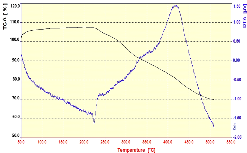
Fig. 5 TGA and DTA curves of the \text{Fe}_3\text{O}_4@CS\text{-TDI-Titriplex V} nanomaterial (1).
