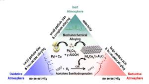
Exploring milling atmosphere effects in mechanochemical synthesis of Pd-Cu supported catalysts for the semihydrogenation of acetylene in equimolar ethylene mixtures
