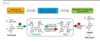
Mechanochemical one-pot synthesis and solid-state transformation of cobalt(II) Schiff base complexes: a green route to tailored coordination architecture
