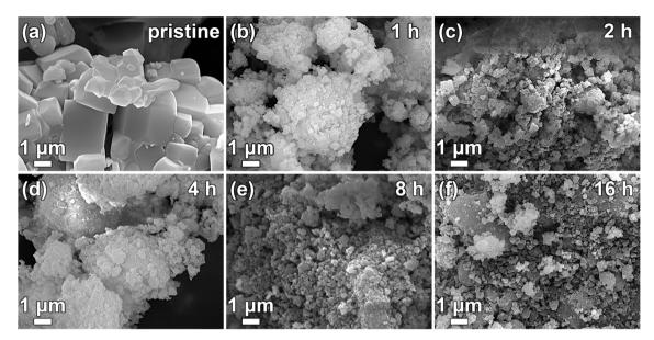
Fig. 3 SEM images of pristine (a) and milled  $NaTi_2(PO_4)_3$  at different milling times with constant rotational speed of 400 rpm, 1 hour (b), 2 hours (c), 4 hours (d), 8 hours (e) and 16 hours (f). Factor of magnification 10 000.
