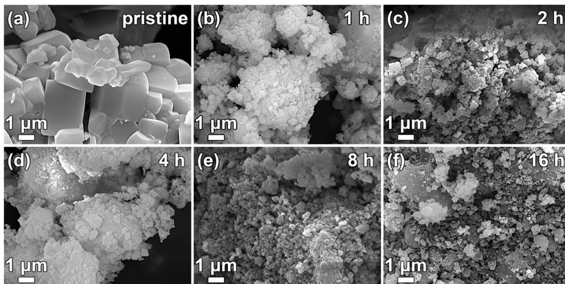
Fig. 3 SEM images of pristine (a) and milled  $\text{NaTi}_2(\text{PO}_4)_3$  at different milling times with constant rotational speed of 400 rpm, 1 hour (b), 2 hours (c), 4 hours (d), 8 hours (e) and 16 hours (f). Factor of magnification 10 000.
