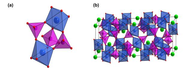
Fig. 1 The lantern unit (a) and the unit cell (b) of a NASICON-structure, shown here using the example of NaTi<sub>2</sub>(PO<sub>4</sub>)<sub>3</sub> (Ti: blue, P: pink, O: red, Na: qreen).
