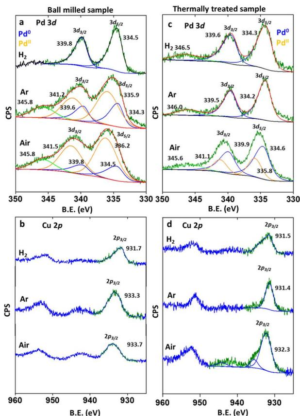
Fig. 4 XPS spectra of 5 wt% Pd<sub>1</sub>Cu<sub>1</sub>/ $\alpha$ -Al<sub>2</sub>O<sub>3</sub> after ball milling in oxidative (air), inert (Ar), reductive (H<sub>2</sub>) atmospheres for Pd 3d (a) Cu 2p (b), and XPS spectra for these samples after thermal treatment for Pd 3d (c) Cu 2p (d).
