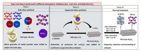
Fig. 1 Schematic illustration for the mechanochemical synthesis of supported Pd-Cu catalysts in oxidative (air), inert (Ar), and reductive (H<sub>2</sub>) environment.
