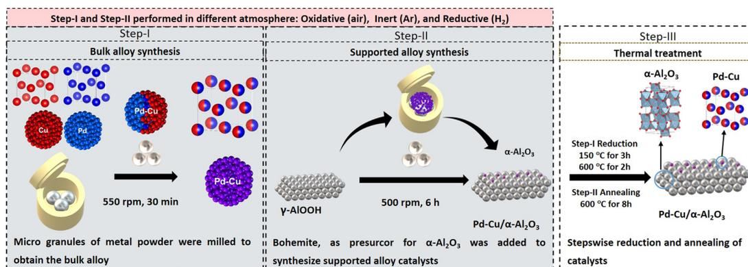
Fig. 1 Schematic illustration for the mechanochemical synthesis of supported Pd–Cu catalysts in oxidative (air), inert (Ar), and reductive ( $\text{H}_2$ ) environment.
