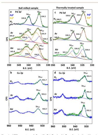
Fig. 4 XPS spectra of 5 wt%  $Pd_1Cu_1/\alpha$ - $Al_2O_3$  after ball milling in oxidative (air), inert (Ar), reductive ( $H_2$ ) atmospheres for Pd 3d (a) Cu 2p (b), and XPS spectra for these samples after thermal treatment for Pd 3d (c) Cu 2p (d).
