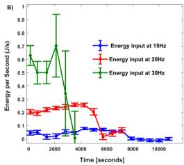
Fig. 8 Knoevenagel condensation reaction. (A) In situ measurement of mean impact force during the reaction using one 12.7 mm stainless steel ball in a stainless-steel jar at 15, 20, and 30 Hz. (B) Mean kinetic energy input on reactant particles towards mechanical activation at different frequencies. For Fig. 8A, mean uncertainty is used rather than the width of the force distribution since using the mean force yields the expected reaction rate (Fig. 7).
