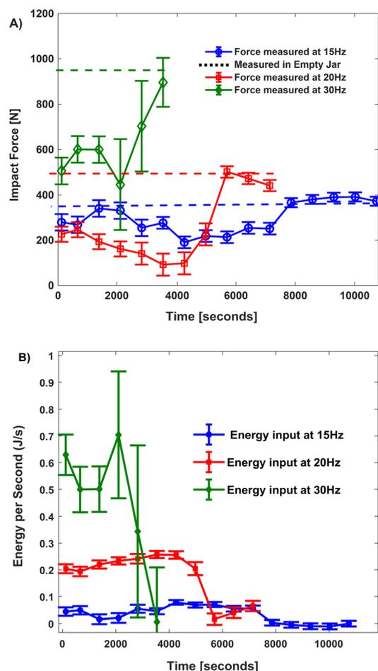
Fig. 8 Knoevenagel condensation reaction. (A) *In situ* measurement of mean impact force during the reaction using one 12.7 mm stainless steel ball in a stainless-steel jar at 15, 20, and 30 Hz. (B) Mean kinetic energy input on reactant particles towards mechanical activation at different frequencies. For Fig. 8A, mean uncertainty is used rather than the width of the force distribution since using the mean force yields the expected reaction rate (Fig. 7).
