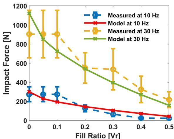
Fig. 3 Impact force measured and modelled as a function of fill ratio for a stainless steel 12.7 mm diameter ball in stainless steel reactor jar at 10 and 30 Hz.
