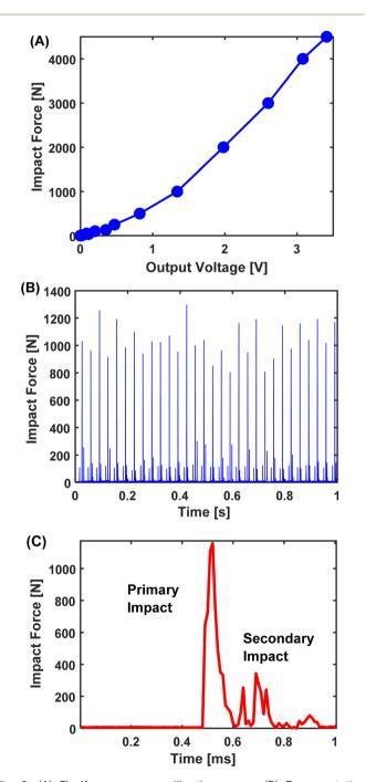
Fig. 2 (A) Flexiforce sensor calibration curve. (B) Representative measurement of impact force using a 12.7 mm SS ball at 30 Hz. (C) Zoomed-in profile of a single impact showing the primary and secondary forces.
