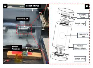
Fig. 1 Schematic of integrated reaction jar. (A) Reactor jar with integrated force measurement in the Retsch MM400. (B) 3D model of the assembled iar featuring the force sensing assembly
