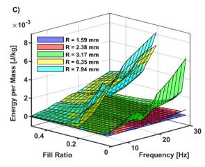
Fig. 6 (A) Measured impact force exerted by the milling ball onto the wall of the reactor jar. (B) Kinetic energy on reactant particles for different ball sizes with varying fill ratios. (C) Specific kinetic energy input on reactant mixture for different ball sizes with varying fill ratio.
