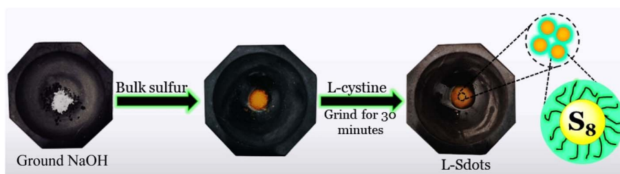
Fig. 6 Illustration of the steps involved in the mechanochemical synthesis of luminescent, chiroptically active L-Sdots using elemental sulfur. Reproduced from ref. 29 with permission from American Chemical Society, copyright 2024.
