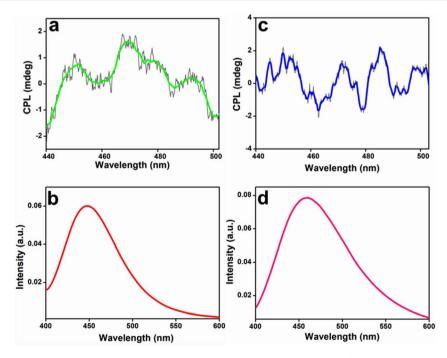
Fig. 10 (a and b) CPL spectrum and the corresponding emission spectrum of L-Sdots respectively, (c and d) CPL and the corresponding emission spectrum of D-Sdots, respectively. Reproduced from ref. 29 with permission from American Chemical Society, copyright 2024.
