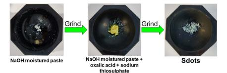
Fig. 5 Illustration of the steps involved in the mechanochemical synthesis of fluorescent Sdots using a mortar and pestle for grinding. Reproduced from ref. 28 with permission from American Chemical Society, copyright 2021.
