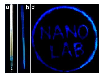
Fig. 15 Sdot-based gel ink filled in the ballpoint pen observed under (a) daylight and (b) UV light of 365 nm, (c) image of the handwriting on non-fluorescent paper under UV light. Reproduced from ref. 29 with permission from American Chemical Society, copyright 2024.
