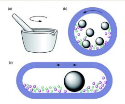
Fig. 1 Schematic representations of the three main modes of mechanical activation of chemical reactions: (a) grinding with a mortar and pestle, (b) planetary ball milling; (c) high-speed vibration milling in a mixer mill. Reproduced from ref. 79 with permission from Royal Society of Chemistry, copyright 2018.
