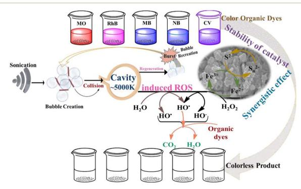
Fig. 12 Mechanism for cavitation-induced dye degradation sonochemically in the presence of mechanochemically synthesized pyrrhotite NPs. Reproduced from ref. 74 with permission from Elsevier, copyright 2022
