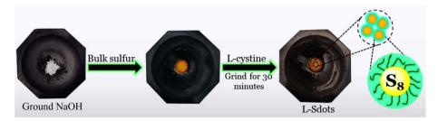
Fig. 6 Illustration of the steps involved in the mechanochemical synthesis of luminescent, chiroptically active L-Sdots using elemental sulfur. Reproduced from ref. 29 with permission from American Chemical Society, copyright 2024.
