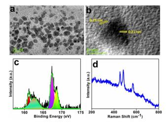
Fig. 7 (a) TEM image of the Sdots, (b) HRTEM image showing the observed d-spacing in Sdots, (c) deconvoluted high-resolution XPS spectrum of the S<sub>2p</sub> region, (d) Raman spectrum of Sdots. Reproduced from ref. 28 with permission from American Chemical Society, copyright 2021.
