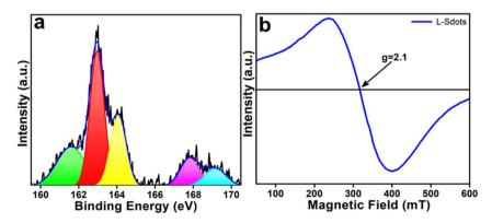
Fig. 8 (a) Deconvoluted high-resolution XPS spectrum of the  $S_{2p}$  region of L-Sdots, (b) EPR spectrum of L-Sdots recorded at room temperature. Reproduced from ref. 29 with permission from American Chemical Society, copyright 2024.
