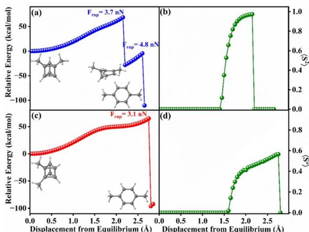
Fig. 1 CoGEF plots at the broken-symmetry UB3LYP/6-31G(d,p) level for (a) pulling across 1,2-positions and (c) pulling across 1,4-positions; the expectation value  $\langle S^2 \rangle$  is given in (b) and (d) respectively.
