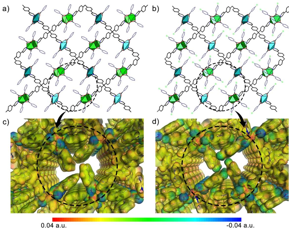
Fig. 4 Comparison between the crystal expansion of (a) **op-TPPM-mCPW(Ph)** and (b) **op-TPPM-mCPW(*p*-FPh)**, followed by their potential electrostatic surfaces (c and d). For both MOFs, the structure has been oriented along the crystallographic *b*-axis. The surfaces have been calculated at the M06-L level of theory using the DMol<sup>3</sup> package of the Materials Studio software.<sup>54</sup>
